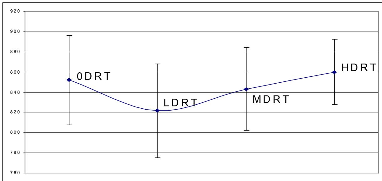
**FIGURE 3:** Flexural strength at various doses. (0D = zero dose, LD = low dose, MD = medium dose, HD = high dose. RT = room temperature)
