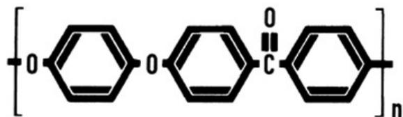
**FIGURE 1:** Chemical structure of poly(aryl ether ether ketone).
