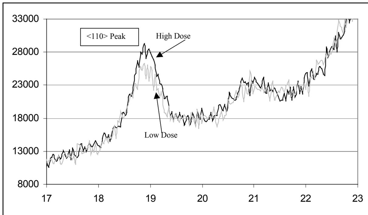
FIGURE 4: Comparison of high dose and zero dose X-ray diffraction patterns.
