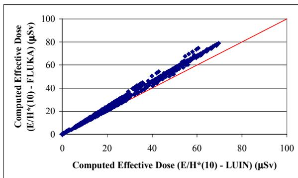
**Figure 3:** Comparison of effective doses as computed using LUIN and FLUKA-based E/H\*(10) scaling ratios.
