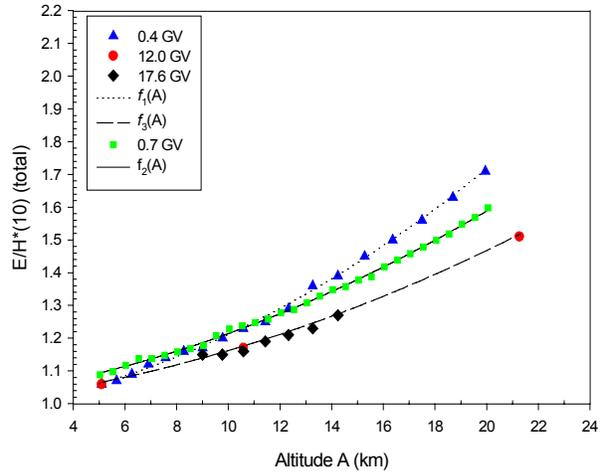
Figure 1:  $E/H^*(10)$  ratio derived from FLUKA calculations.
