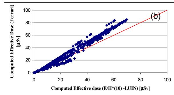
**Figure 4:** Comparison of effective doses as computed by Ferrari's model and the (a) E/H\*(10)<sub>FLUKA</sub>, and (b) E/H\*(10)<sub>LUIN</sub> ratios.
