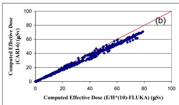
**Figure 5:** Comparison of effective doses as computed by CARI-6 and the (a) E/H\*(10)<sub>FLUKA</sub>, and (b) E/H\*(10)<sub>LUIIN</sub> ratios.
