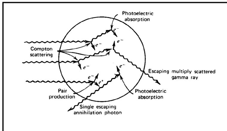
**Fig. 3: Intermediately sized detector**
