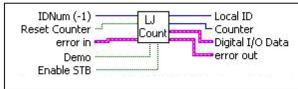
**Figure 5-1: The function of “Count” for communicating between the CNT port of the LabJack and the LabVIEW code.**
