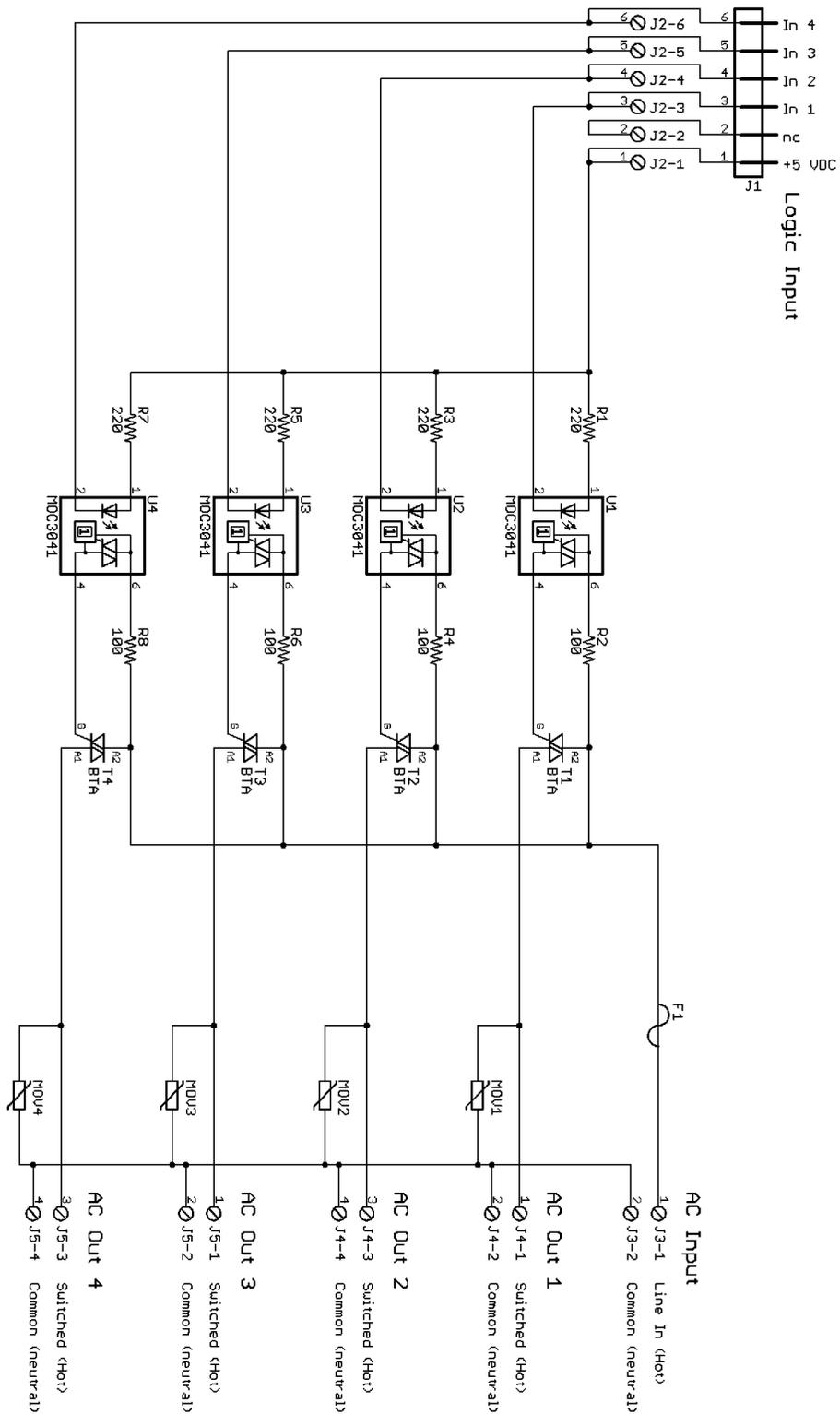
Figure 3-8: Schematic picture of Triacout4
