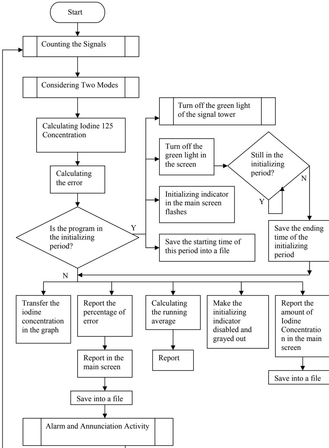
Figure 4-5: The detail of “calculating the Iodine Concentration and demonstrating the result” in the overview flowchart.
