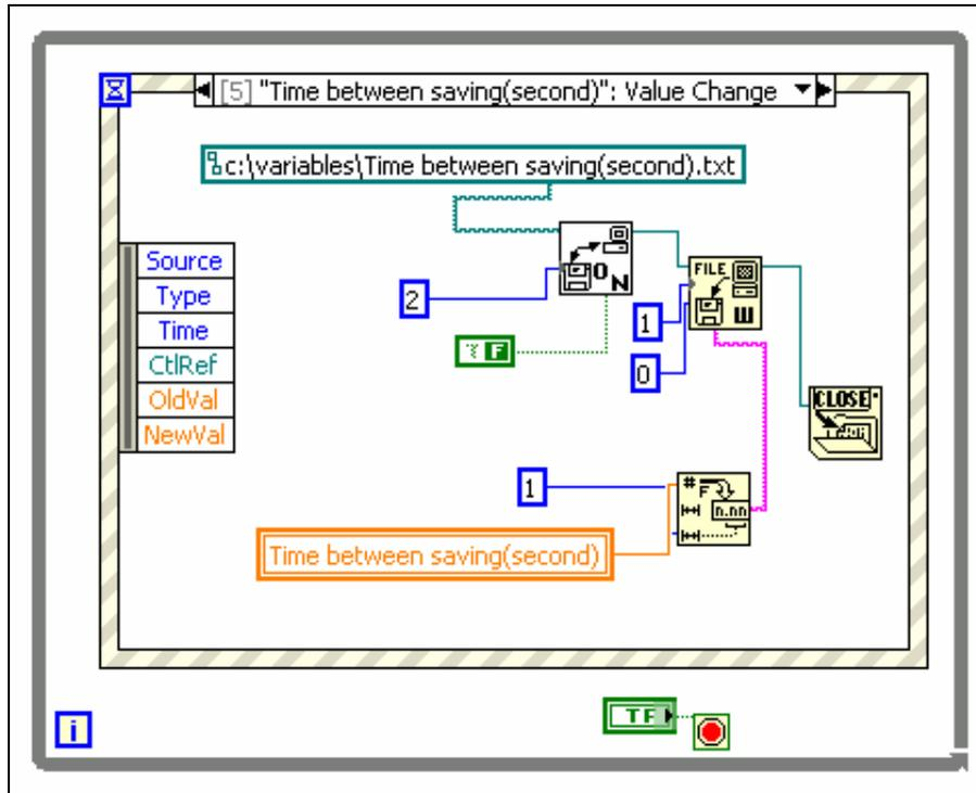
Figure 5-51: The old value of “Time between saving (second)” is replaced by the new one if the operator changes its value when the program is running.
