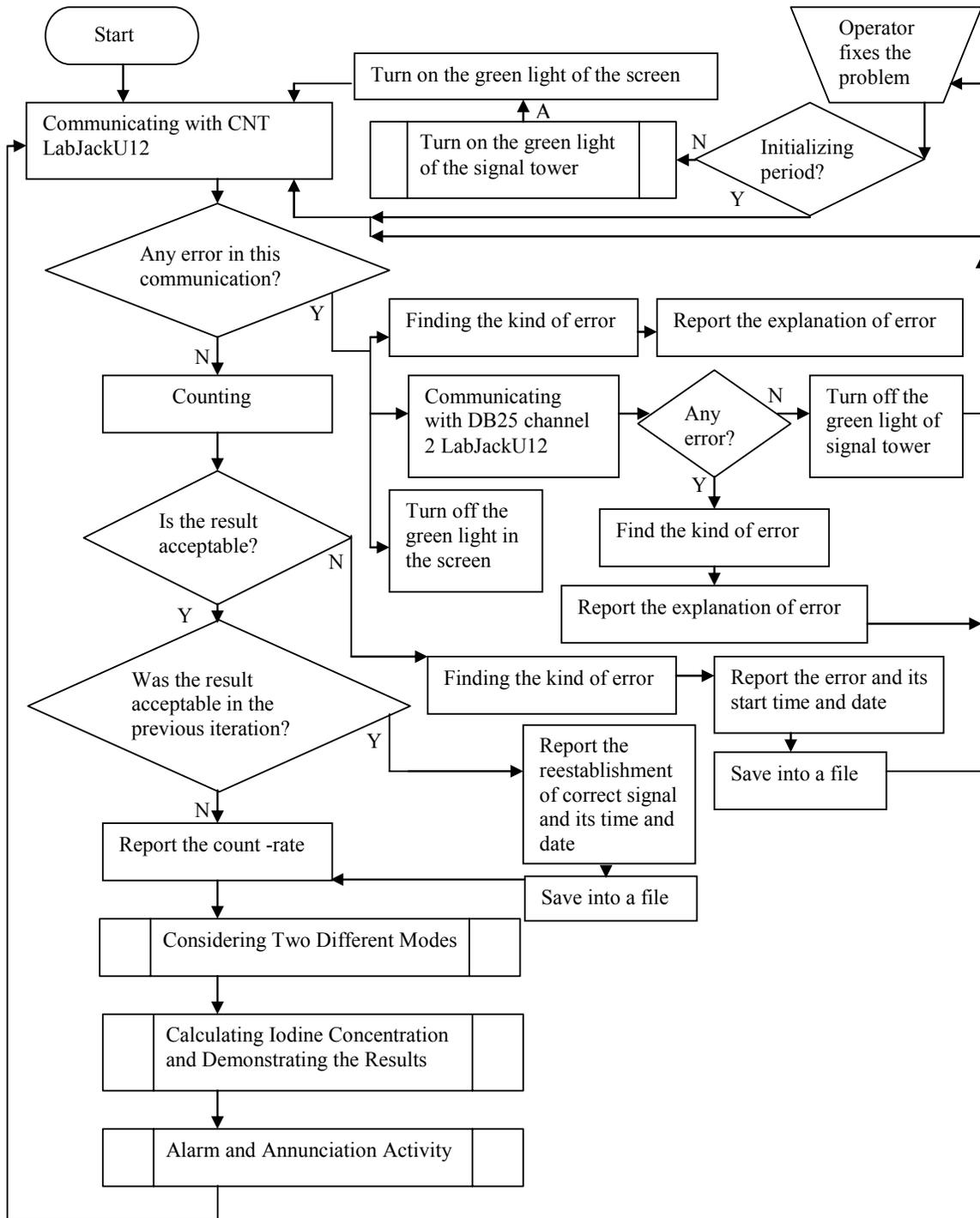
Figure 4-2: Detailed process of the “Counting the Signals” in the overview flowchart.
