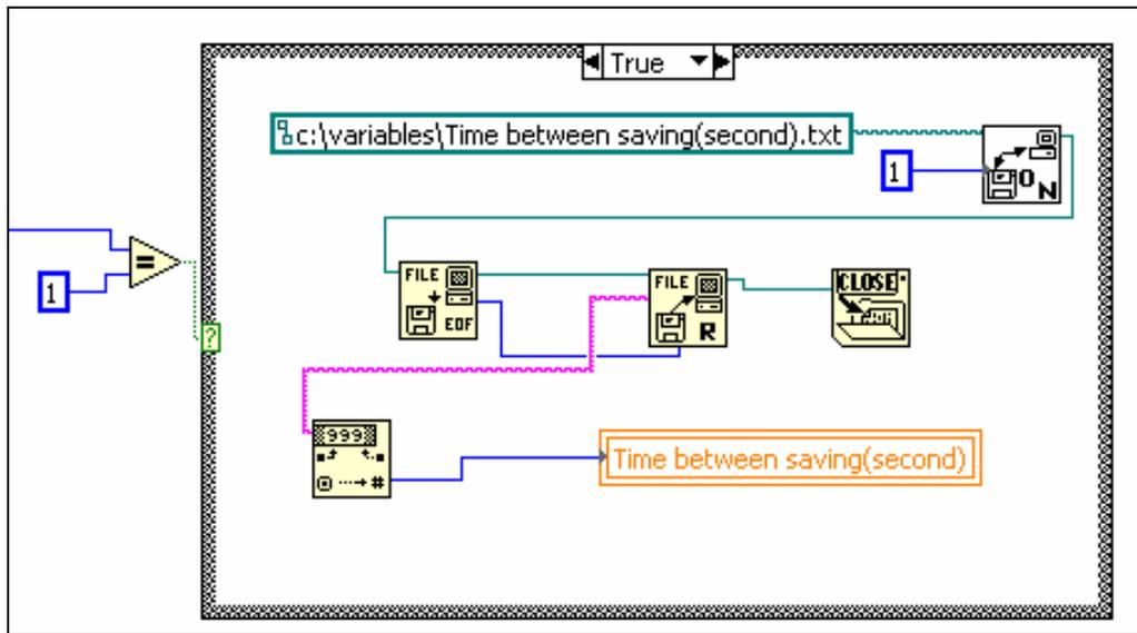
Figure 5-54: At the iteration #1 (second iteration), the variable of "Time between saving (second)" read the value saved in the corresponding file.
