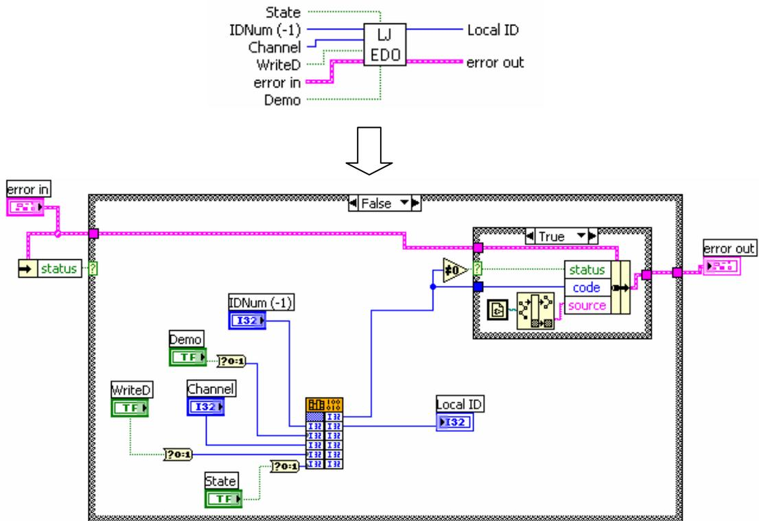
**Fig. VIII :** The code of “EDigitalOut”. The other cases of the both case structures contain nothing only connections between “error in” and “error out”.
