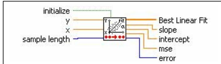
Figure 5-22: The function of “Linear Fit PtByPt”.
