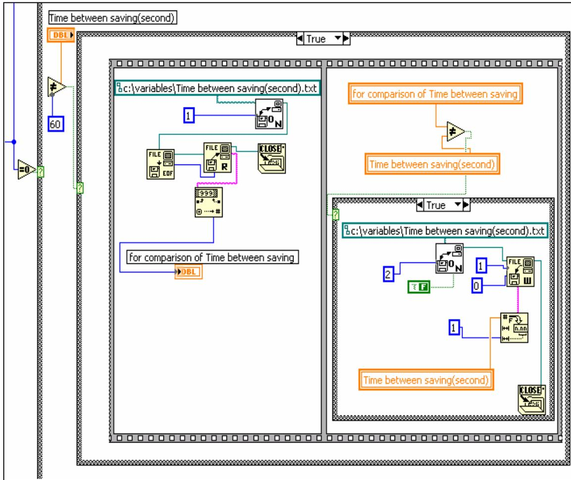
Figure 5-55: This process runs in iteration #0, i.e. the first iteration. It is designed for the situation that the operator changes the value of a variable when the program is not running, and therefore, the new value is not saved in the file.
