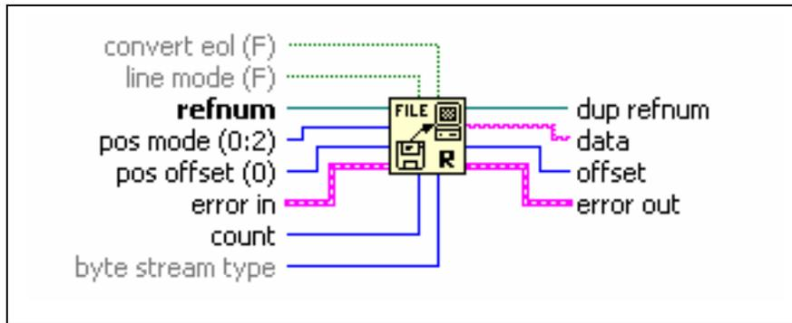
Figure 5-52: The “Read file” used in the reading process from a file.
