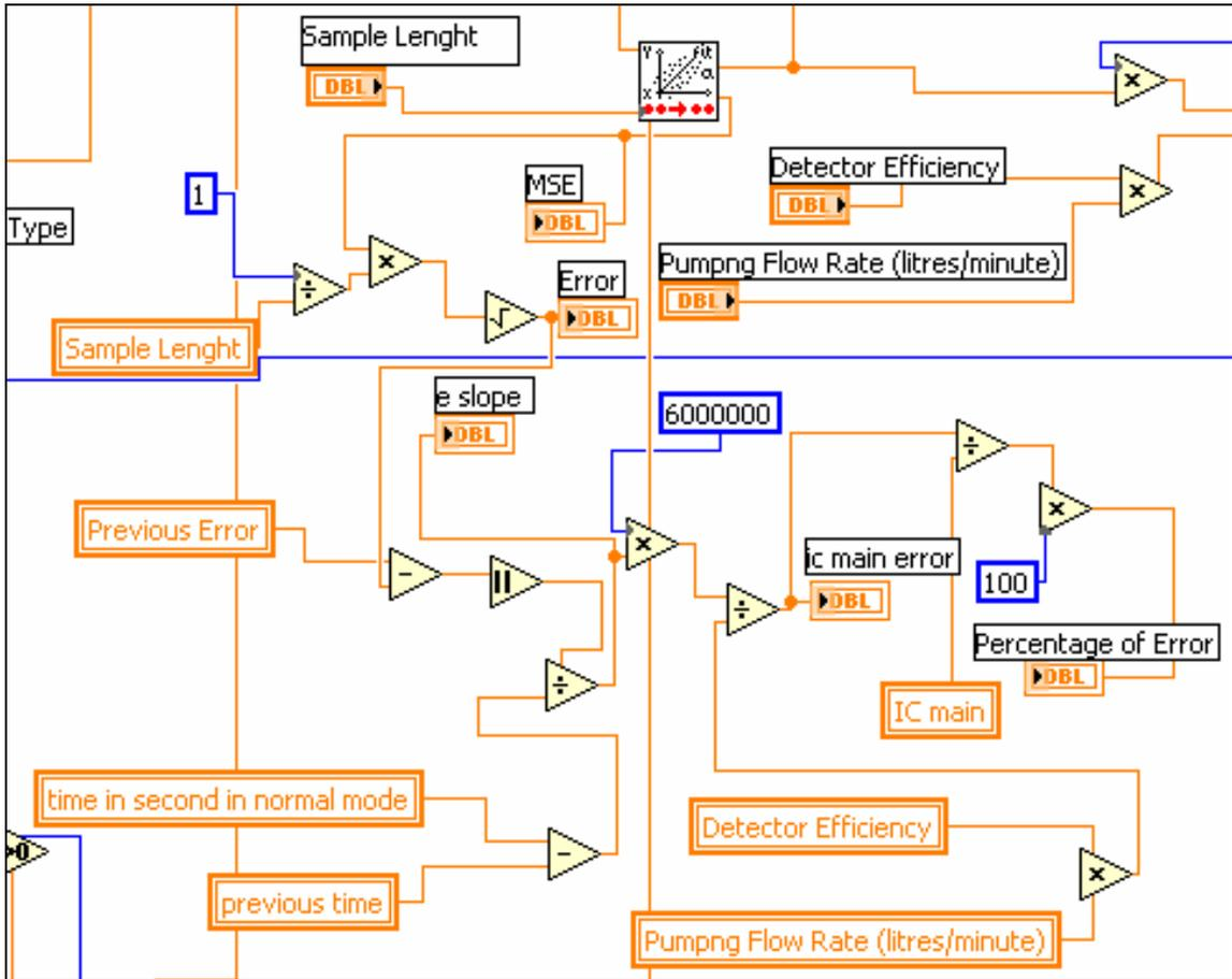
Figure 5-24: The Percentage of Error is calculated in this part of the code.
