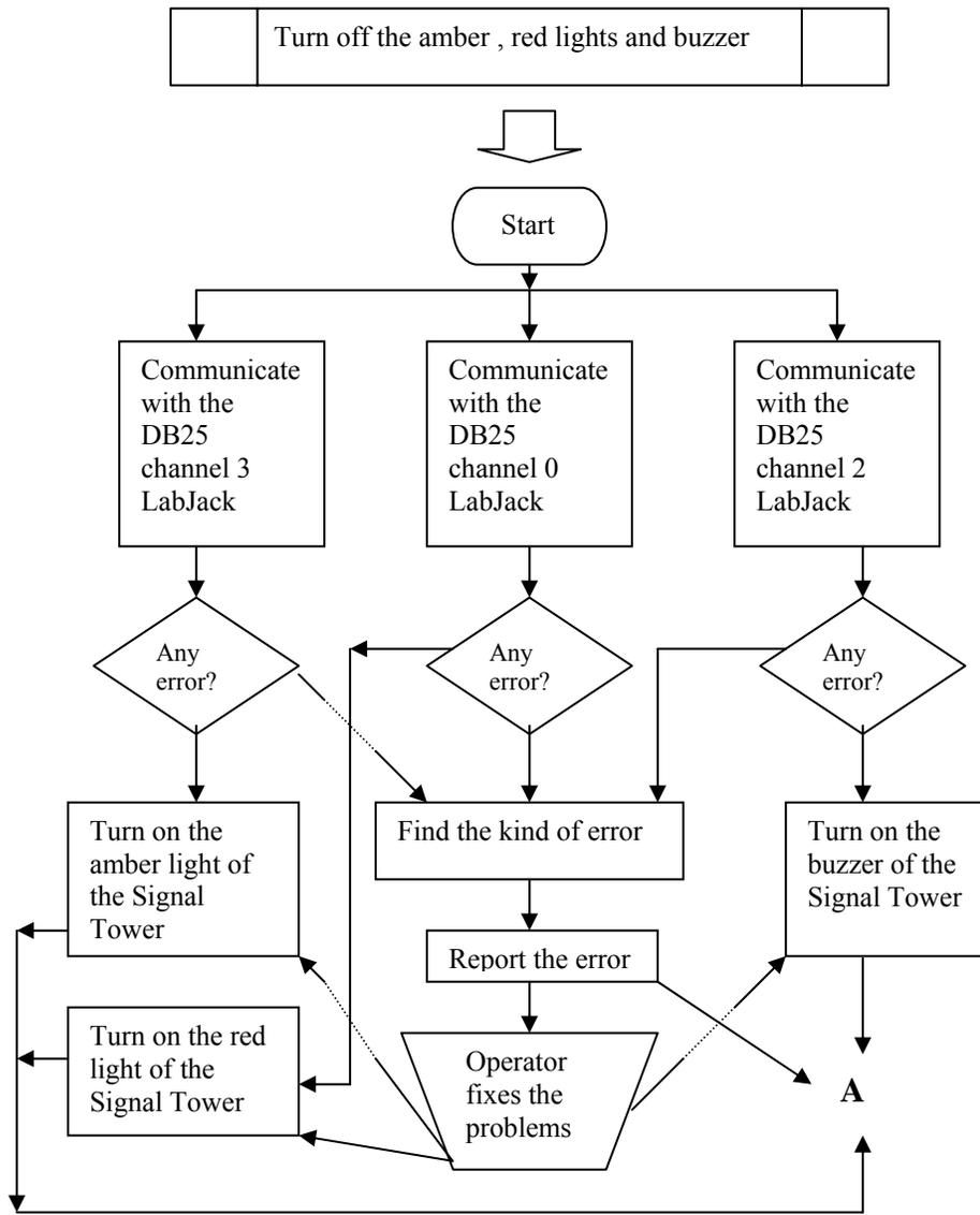
Figure 4-7: Definition of “Turn off the amber, red lights and buzzer”
