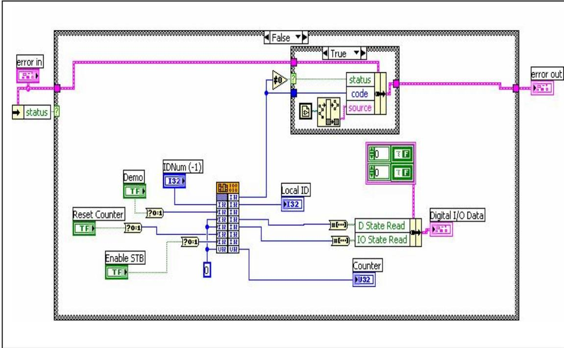
**Figure 5-2: Block Diagram of the sub-VI "Count". Other cases of the case structures are empty. They are just connections between "error in" and "error out".**
