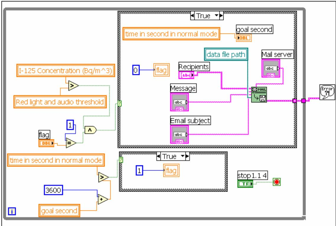
Figure 5-36: Part of the code responsible for sending email to the crew of the reactor at the time of the alarm situation. The daily data file is attached to this email. The frequency of sending the email is one hour.
