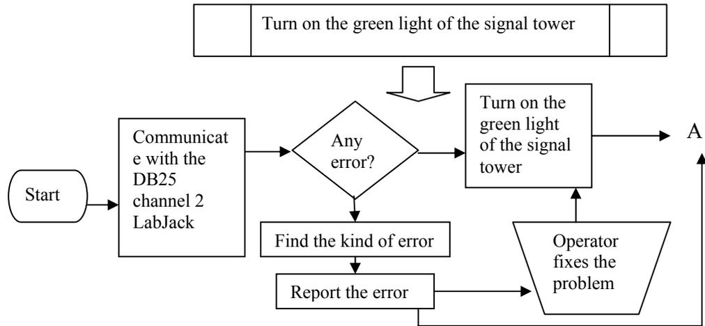
Figure 4-3: “Turn on the green light of the signal tower “is defined as above.
