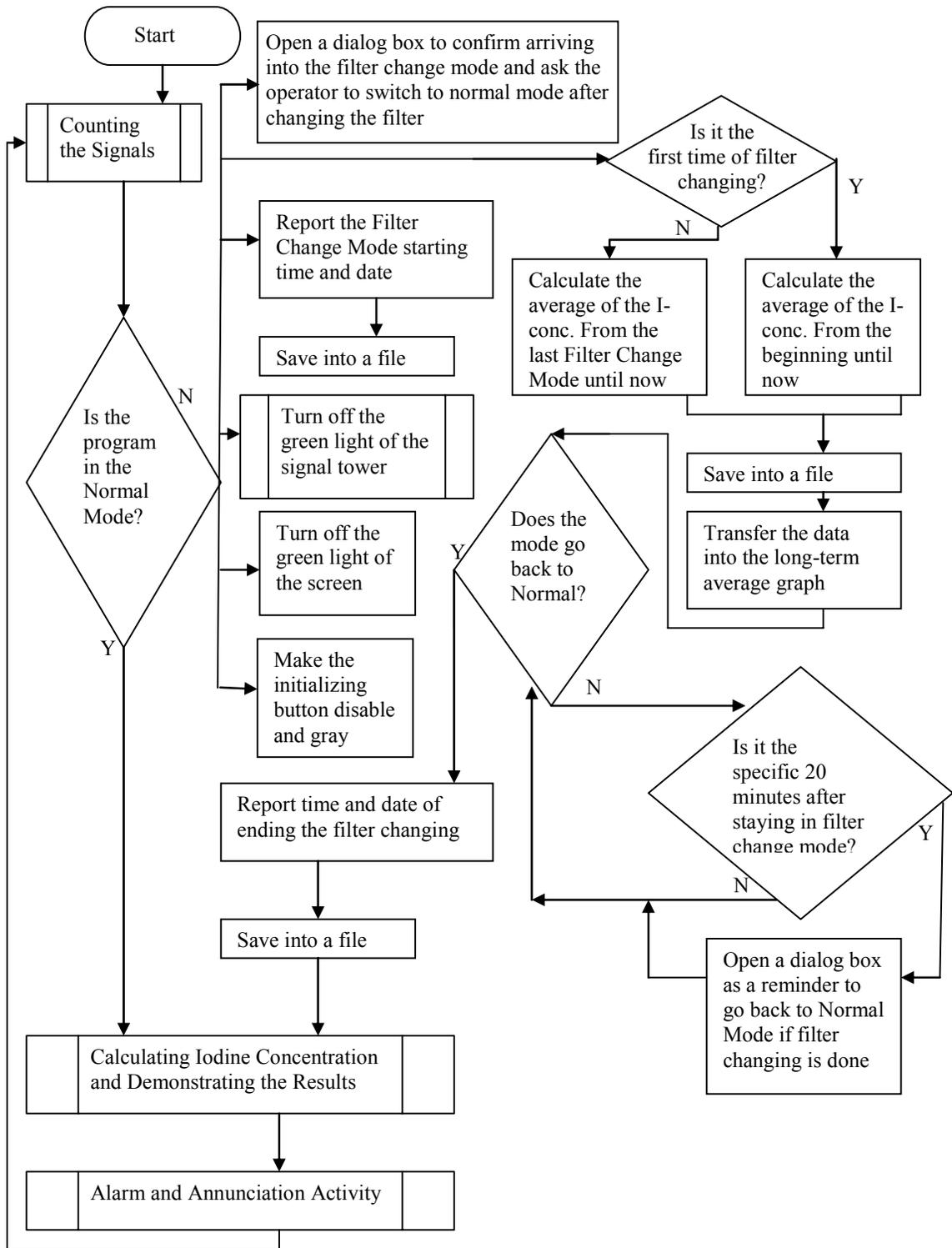
Figure 4-4: Details of the “Considering Two Modes” is shown in this flowchart.
