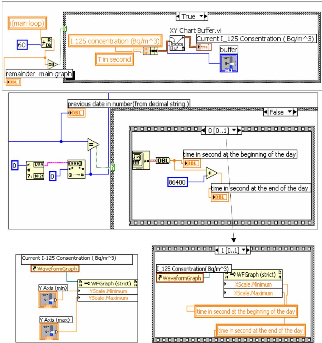
Figure 5-57: Parts of the code that control the “Current I-125 concentration (Bq/m<sup>3</sup>)”graph and transfer the data into it.
