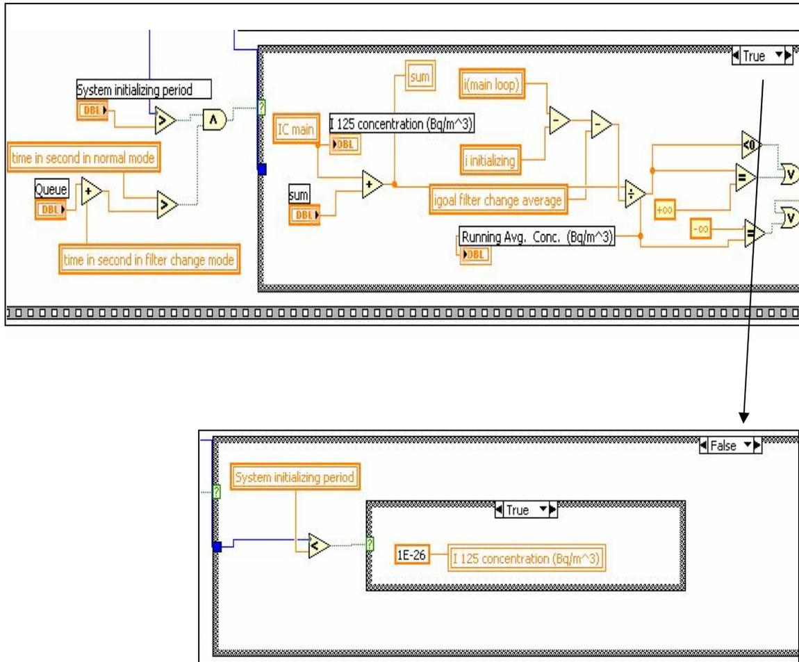
**Figure 5-23:** This part of the main code shows when “IC main” calculated in Figure 5-21 is equal to “I-125 Concentration (Bq/m<sup>3</sup>)”. Also this figure shows how the “Running average” of Iodine Concentration is calculated.
