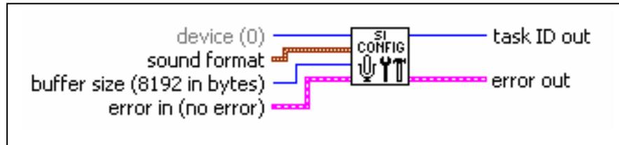
**Figure 5-9 : The appearance of “SI CONFIG”, the first function that is used to communicate with the soundcard of the PC.**
