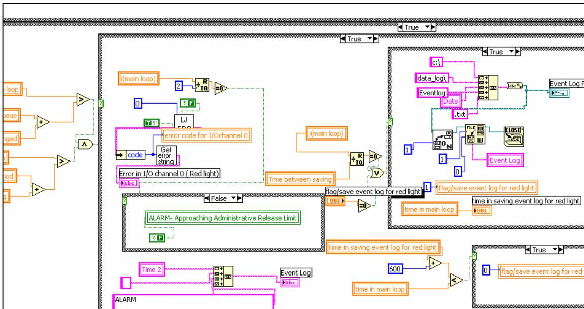
Figure 5-31: This part of the code corresponds to the flashing red light of the signal tower and the screen.
