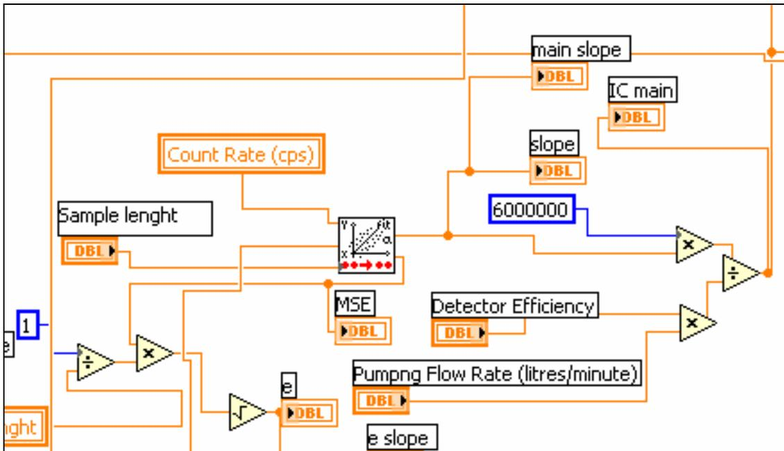
Figure 5-21: The part of the code that shows how Iodine Concentration is calculated. More detailed description of this figure is given in Appendix6
