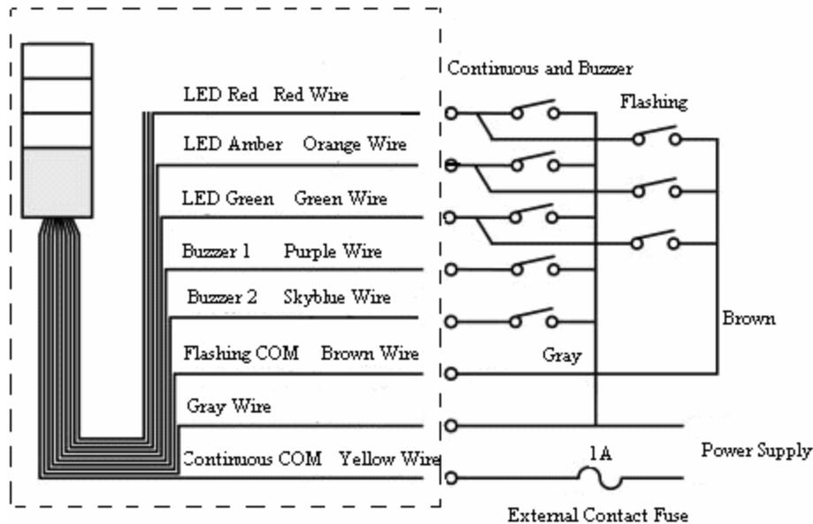
Figure 3-6: Wiring diagram of the signal Tower<sup>6</sup>
