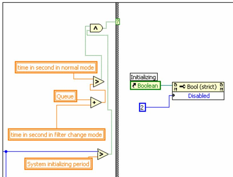
**Figure 5-28: The indicator is disabled and grayed out outside the initializing period.**
