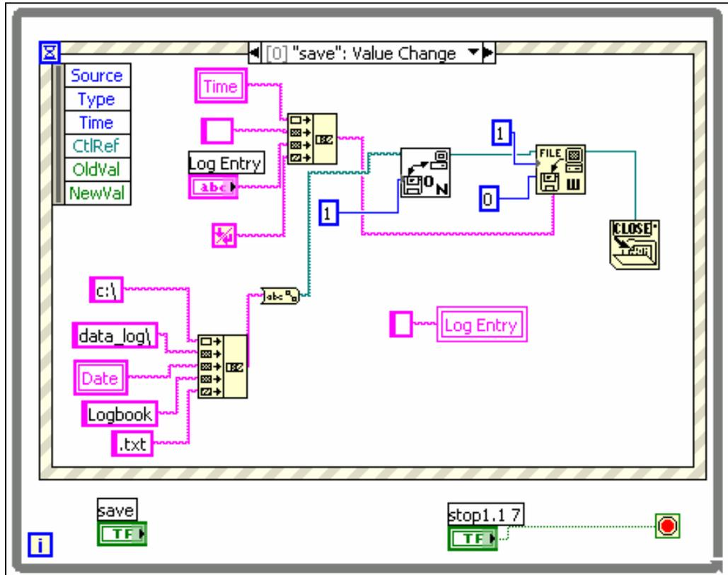
Figure 5-50: This code shows these processes: 1) Creation of a “Logbook” file or opening an existed file. 2) Then saving the content of “Log Entry” box into this file. 3) At last clearing this box.
