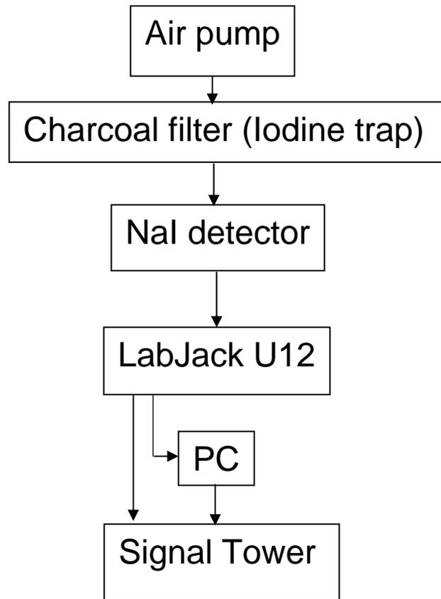
Figure 3-3-1: Main parts of the system hardware
