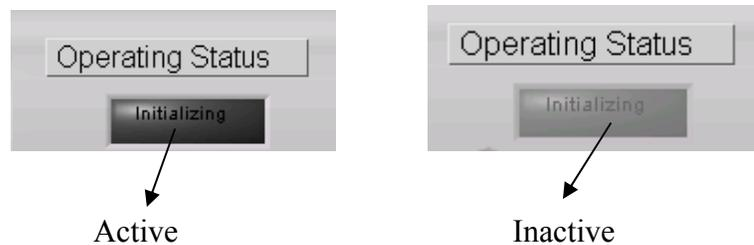
**Figure 5-26: The initializing indicator in the main screen. It flashes, when it is active and it is disabled and grayed out in the inactive duration.**
