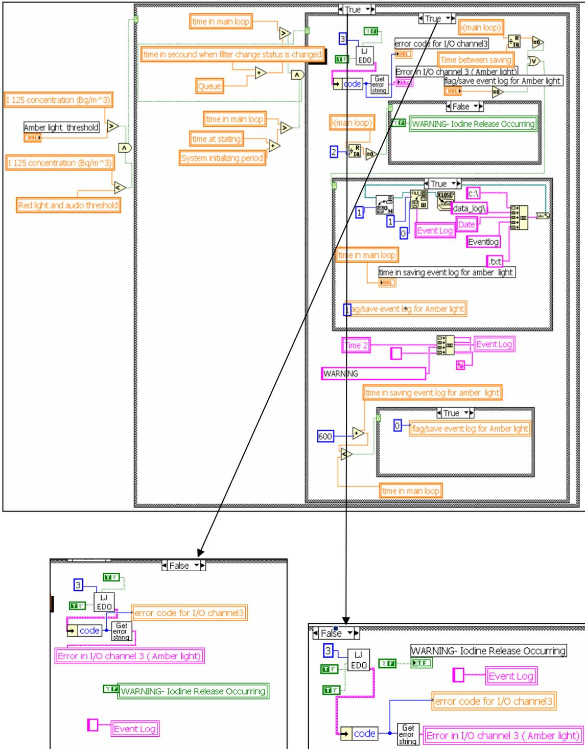
Figure 5-30: This figure shows how the program controls the signal tower amber light and the amber light of the screen.
