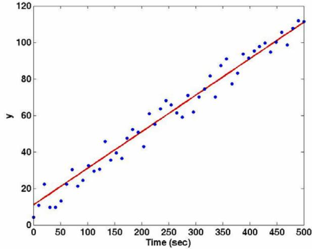
**Figure 2-2-2: Typical experimental data in 500 seconds and the best-fitted line approximated by least-square solution.**
