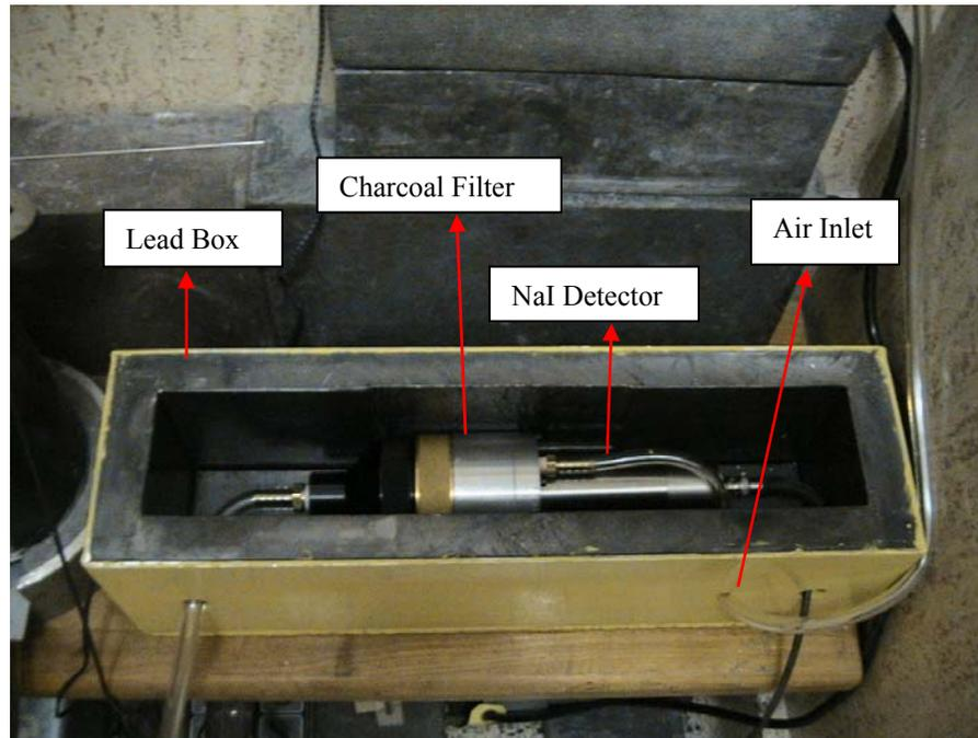
Figure 3-3: NaI Detector and Charcoal Filter in the Lead Box
