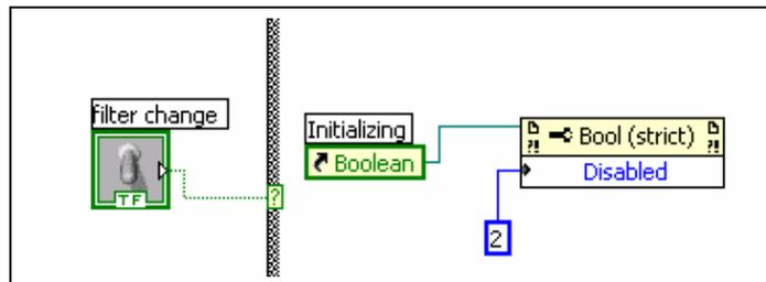
**Figure 5-17: In the Filter Change Mode the indicator of initializing phase is inactive. The case structure is in the “True” case at this figure.**
