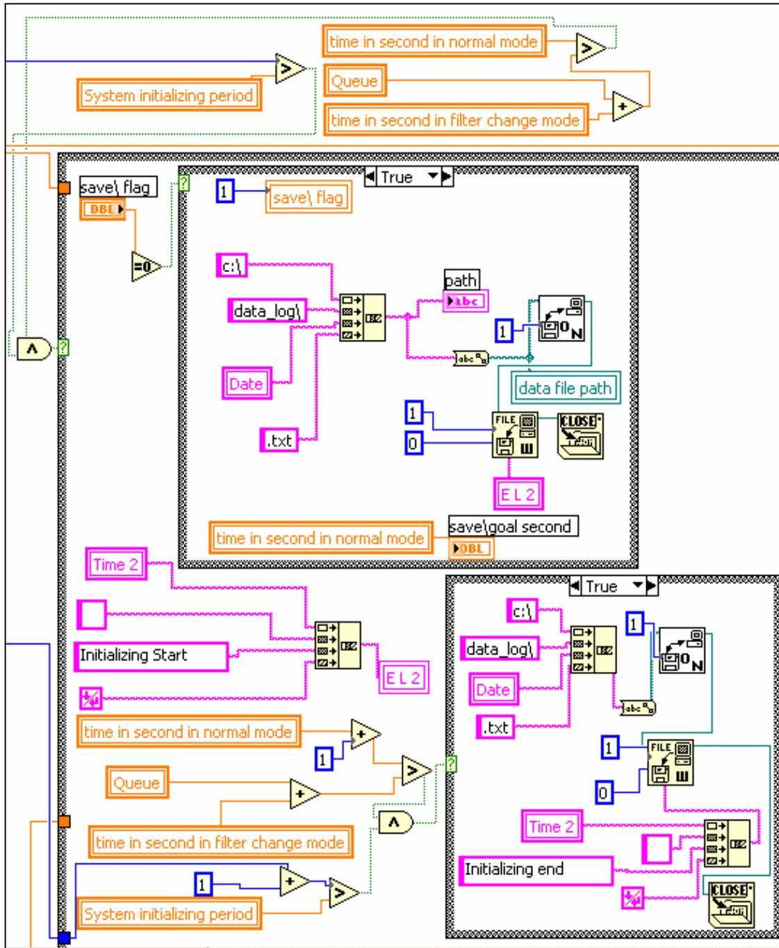
Figure 5-25: The part of the code for reporting of arriving into and exiting from the initializing phase.
