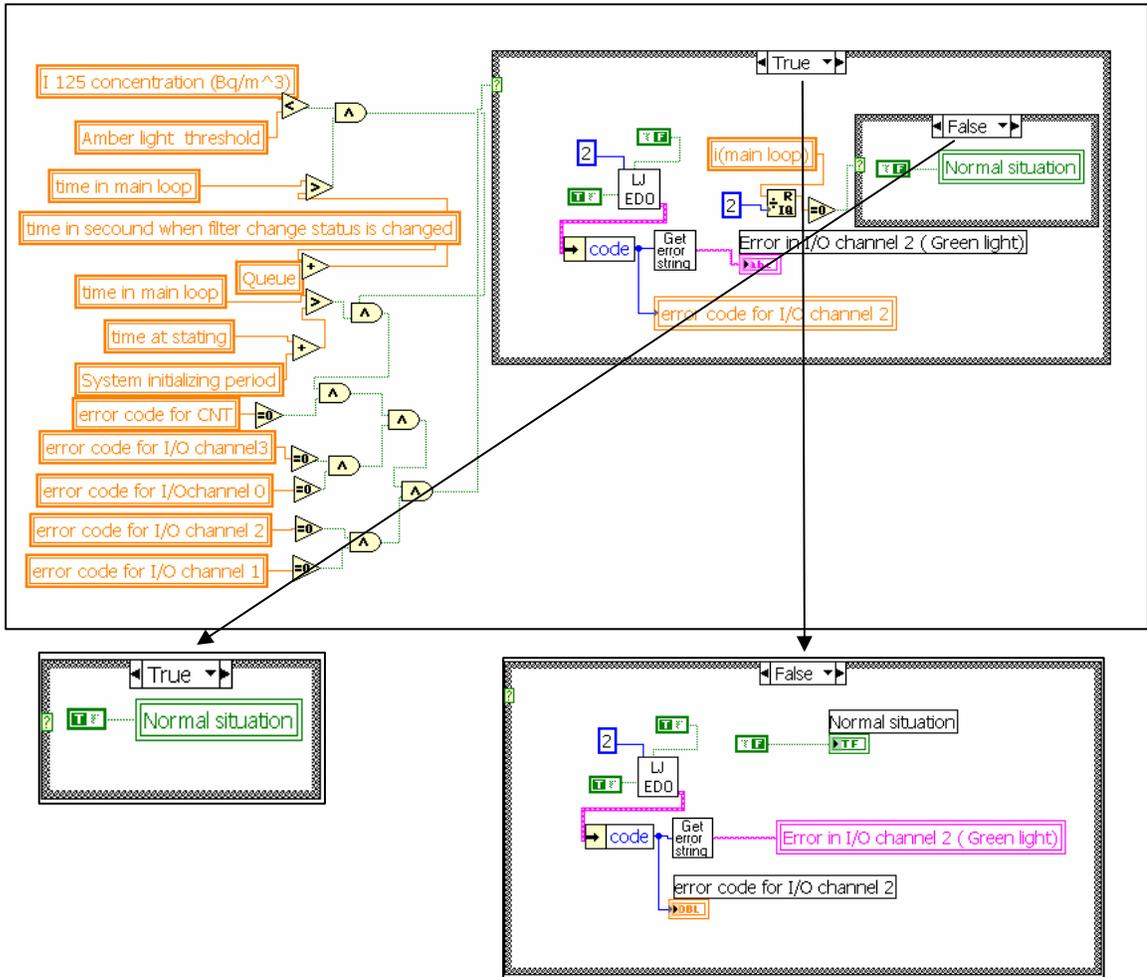
Figure 5-29: Controlling the Signal Tower green light and the green light of the main screen.
