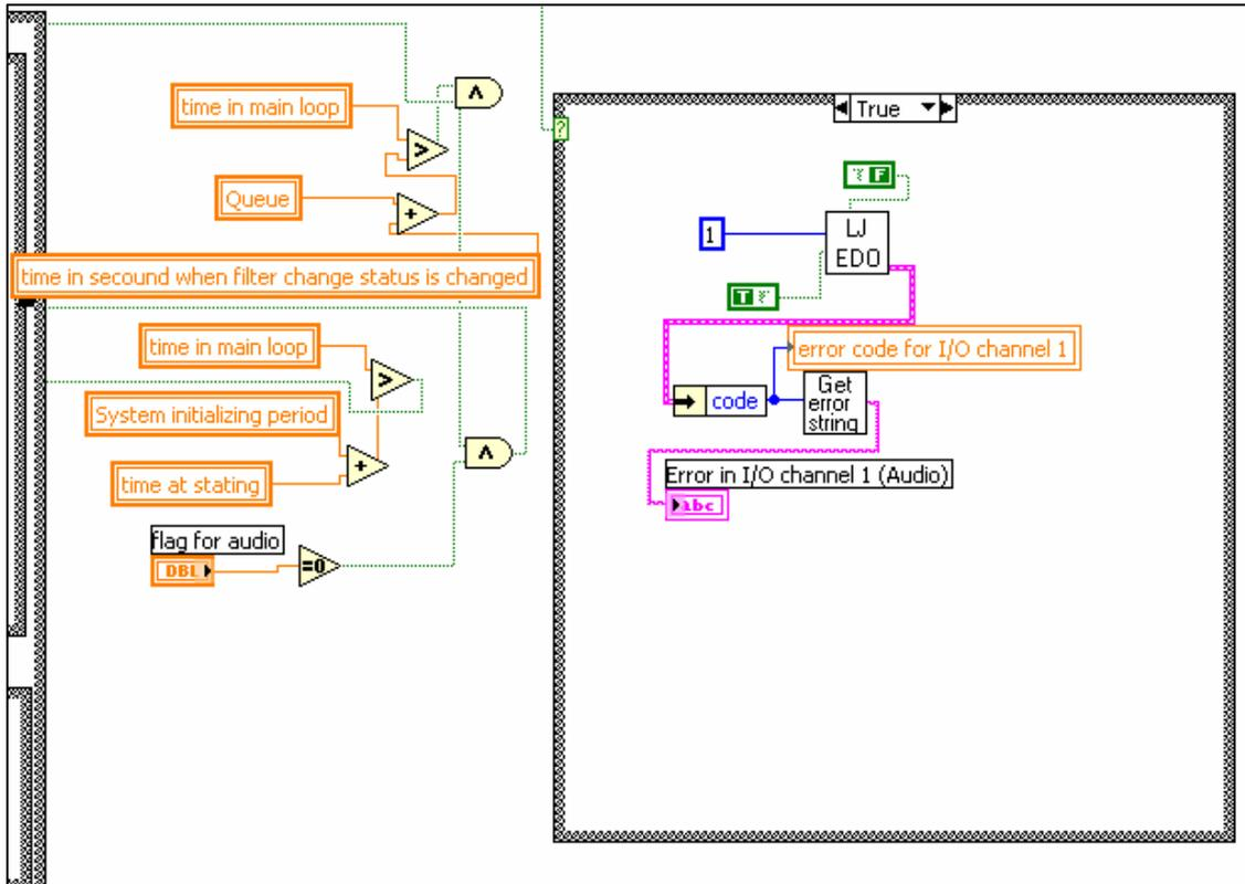
Figure 5-32: Controlling the buzzer of the Signal Tower.
