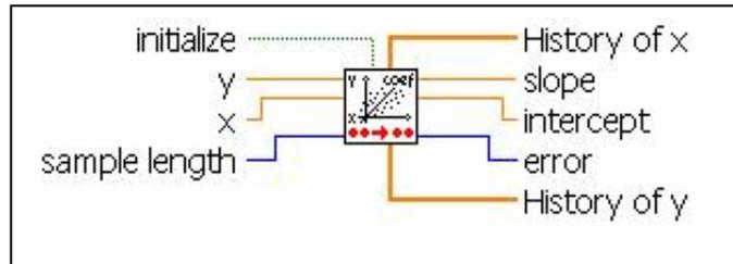
Fig. III: “Linear Fit Coefficients PtByPt”.
