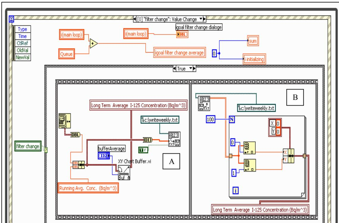
Figure 5-59: Part of the code related to the data transferring into the graph of “Long Term Average I-125 Concentration (Bq/m<sup>3</sup>)”
