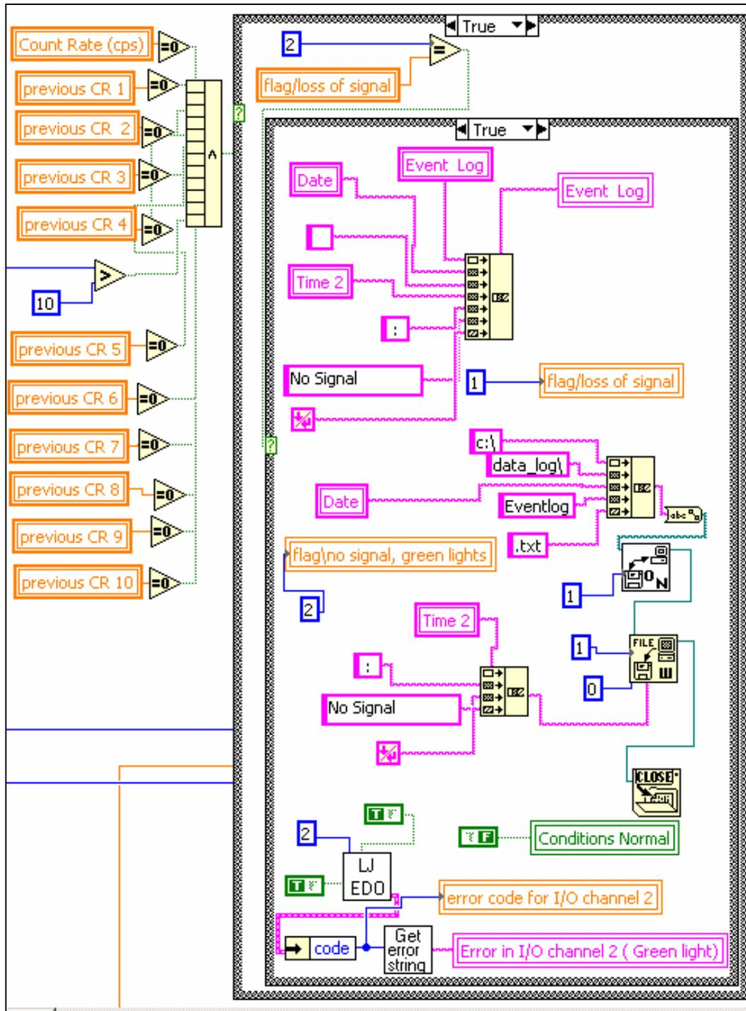
Figure 5-5: When the count-rate is continuously zero, the “NO Signal” error will be reported in the “Event log” box and saved in the “\*eventlog.txt” file.
