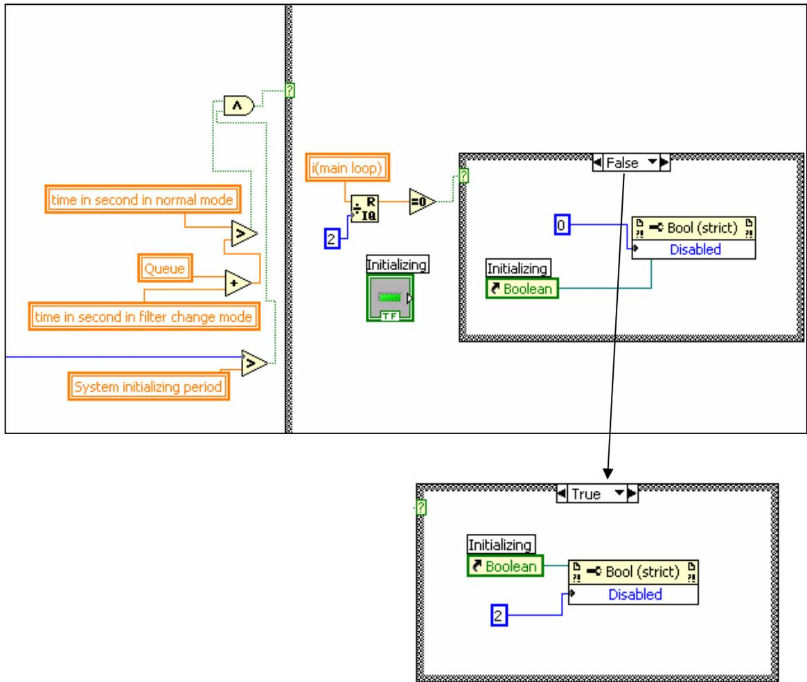
Figure 5-27: When the program is in the initializing period, the initializing indicator flashes.
