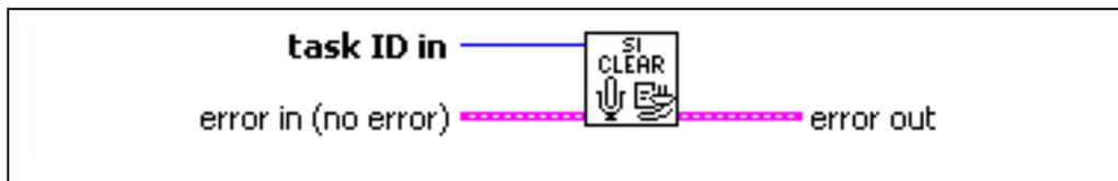
Figure 5-12: The function of “SI CLREAR” to close the sound input device.
