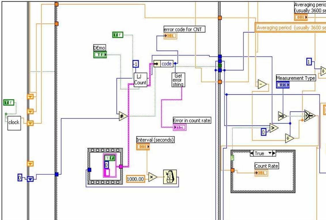
Figure 5-4: Main part of counting section in the MASIS code.
