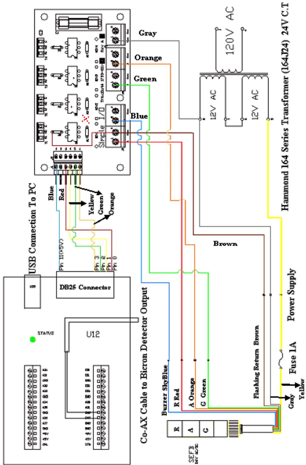
Figure 3-11: Wiring schematic between LabJack U12, TriacOut4, Signal Tower and transformer
