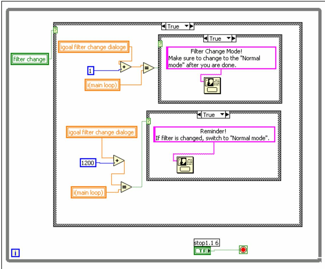
Figure 5-18: The code of the dialog boxes in the separate while loop.
