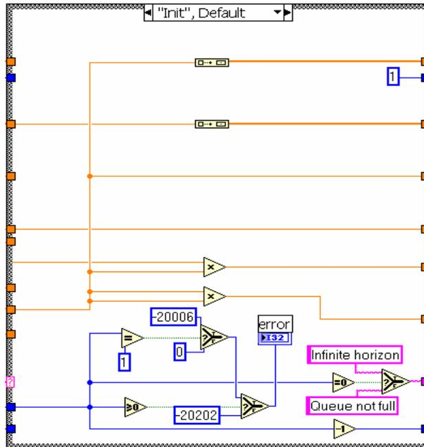
Fig. V: “Linear Fit Coefficients PtByPt”. This code shows how Least Square Solution is employed to find the slope and intercept of the best linear fit. The sequence of the sub-diagrams in the Stacked Sequence Structure is: 1) “Queue not filled” 2) “Finite horizon” 3) “Infinite horizon” 4) “Init, Default”.
