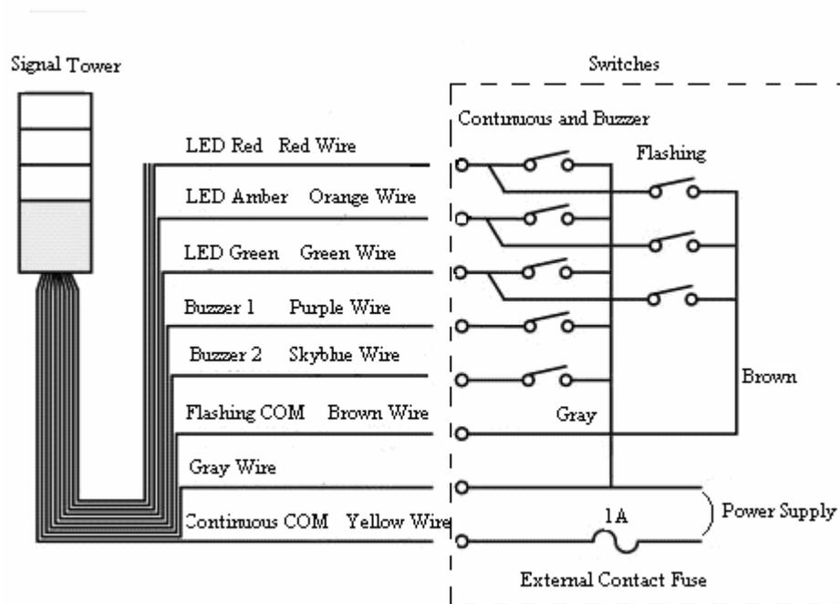
**Figure 3-9: The common wire for flashing is different from the common wire of continuous lights and buzzer.**
