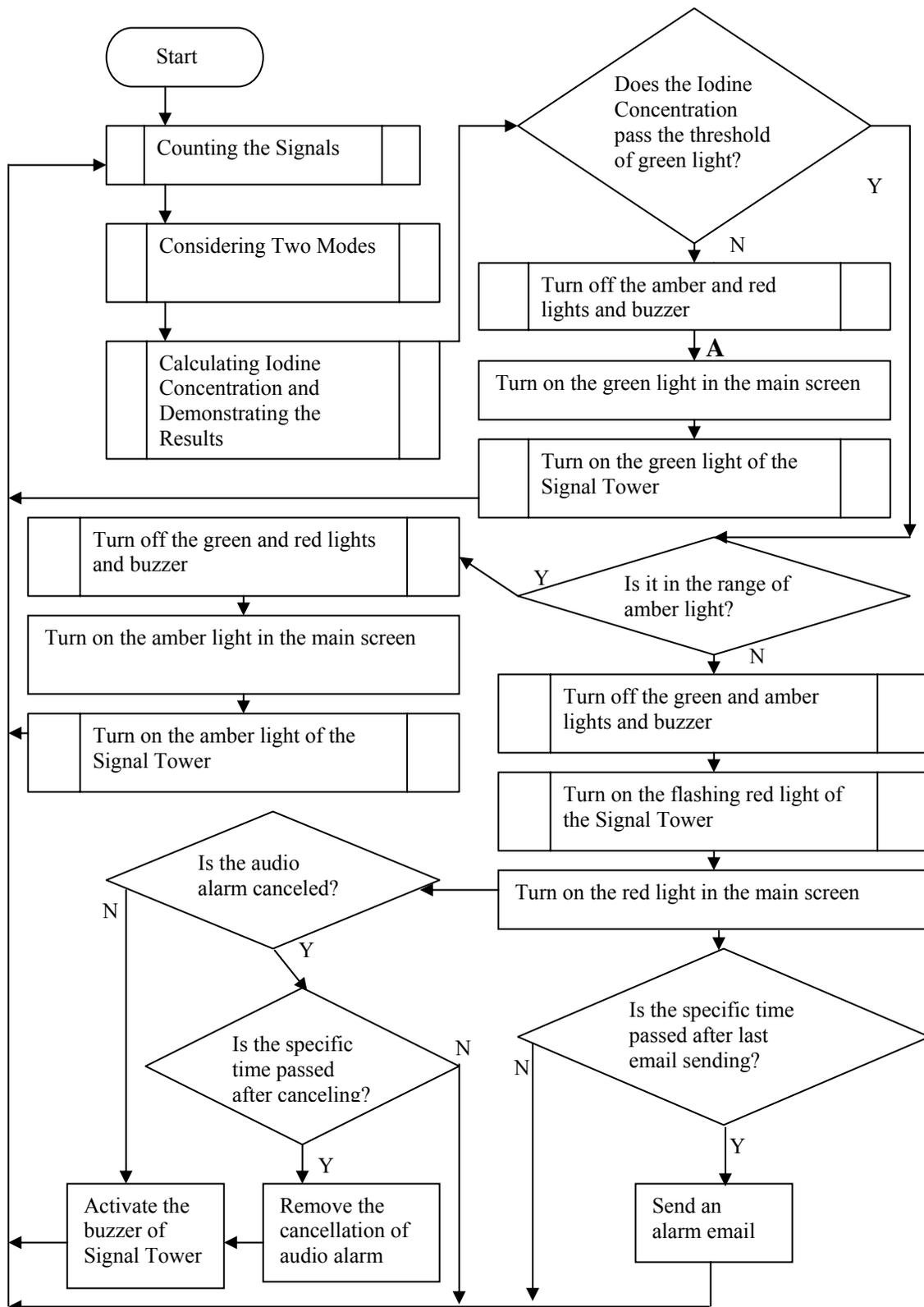
Figure 4-6 : The flowchart of the Alarm and Annunciation System in the overview flowchart.
