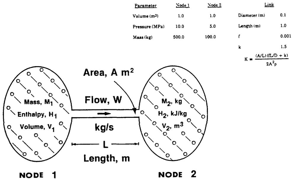
**Figure 5.1** Simple 2-node, 1-link system.
