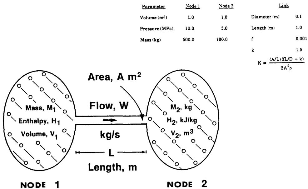
**Figure 5.1** Simple 2-node, 1-link system.
