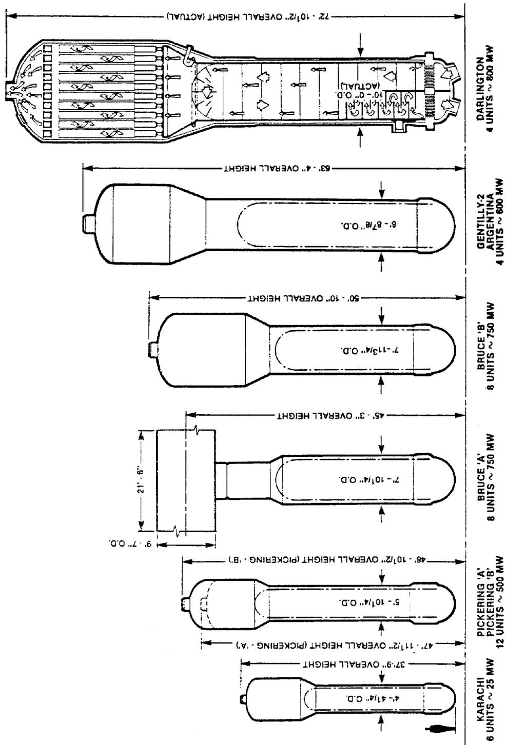
Figure 8.5 Steam generators - relative sizes
