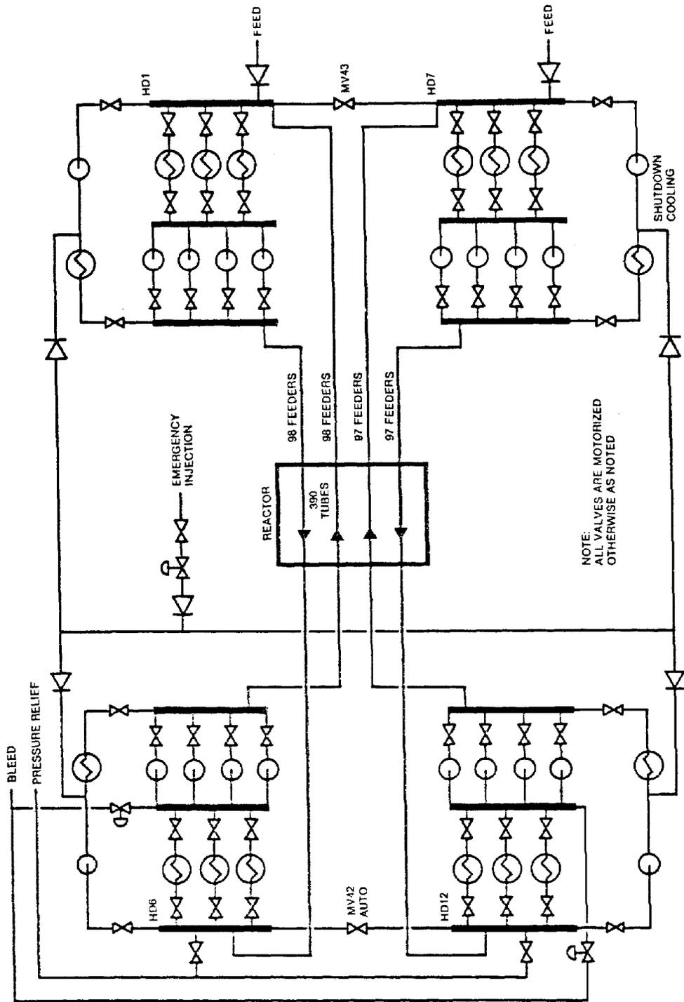
Figure 8.3 Pickering PHT circulating system
