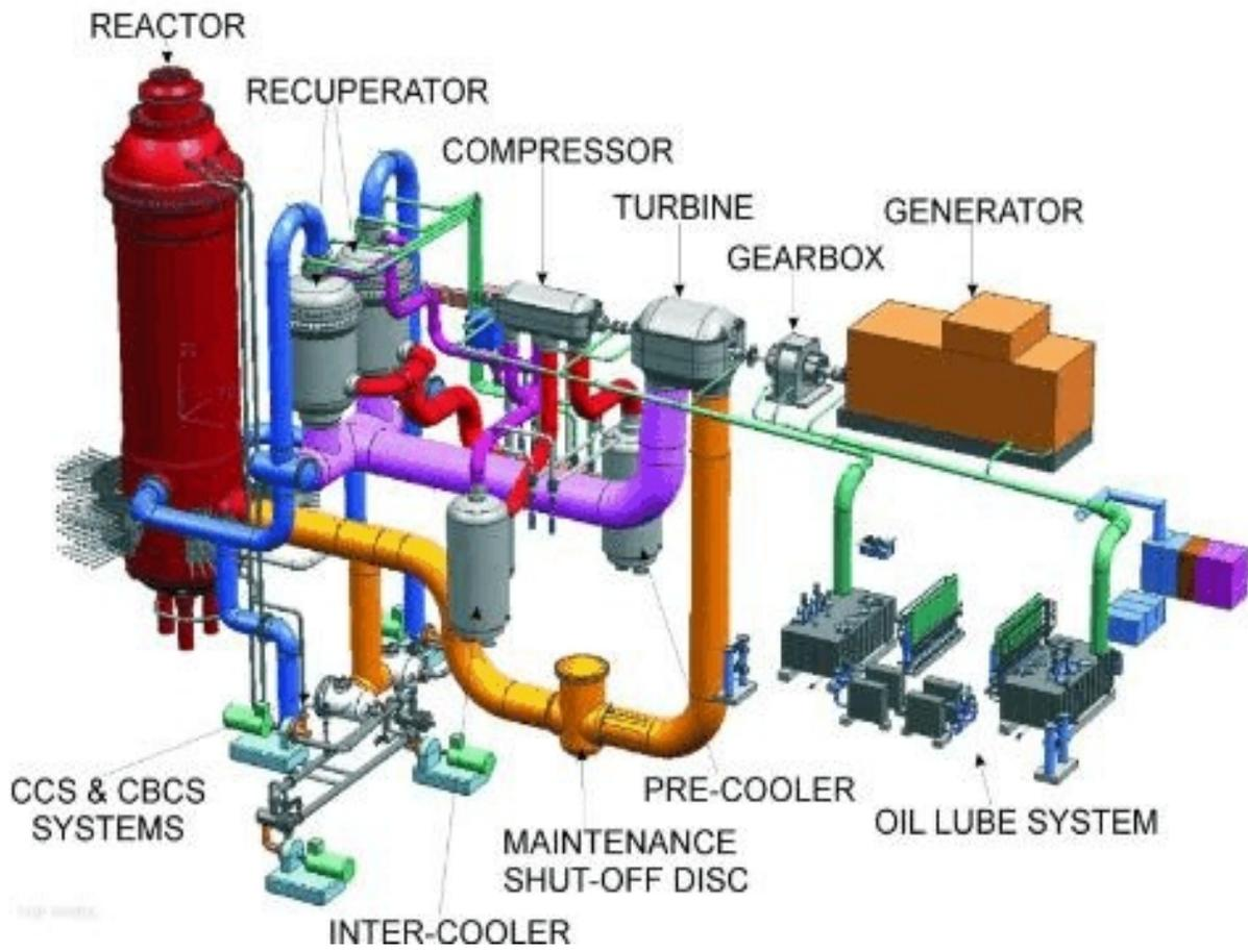
Figure 9b-5 - MPS Layout
