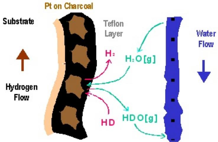
Figure 9b-2 - Hydrogen Recombination via Catalyst
