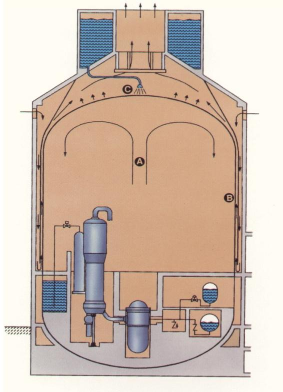
Figure 9b-4 - AP-600 Containment Heat Removal
