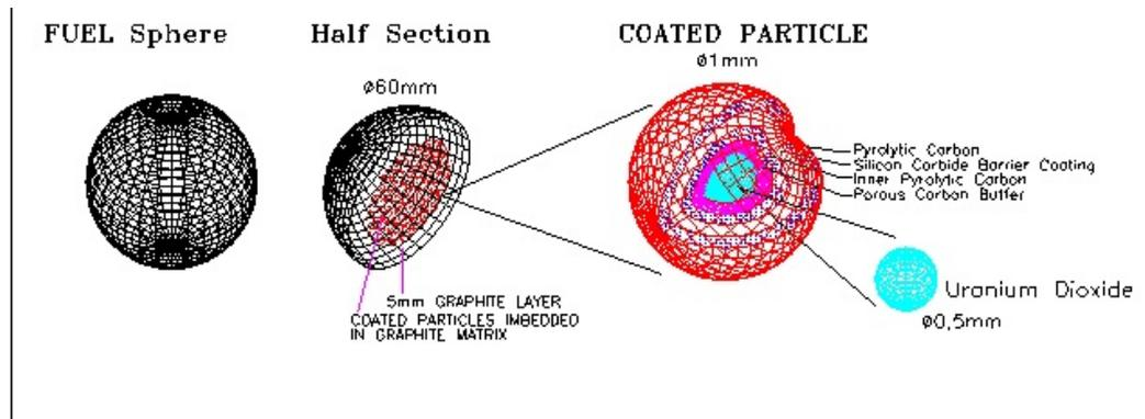
Figure 9b-7 - PBMR Fuel Particle
