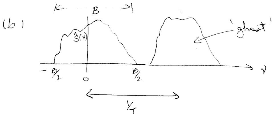
The sampling rate  $1/T$  must be large enough to prevent overlap of the ghost & the signal.
