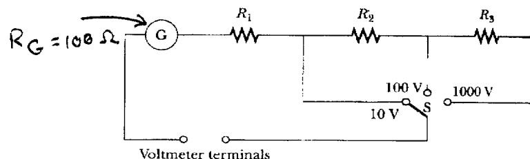
When the switch is in the 10 V position, get 1 mA full scale, i.e 1 mA at 10 Volts.
