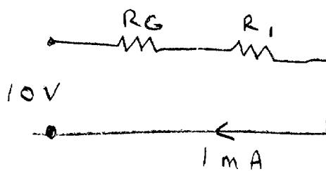
$$\therefore 10 = (R_G + R_1)(0.001) = (100 + R_1)(0.001)$$
