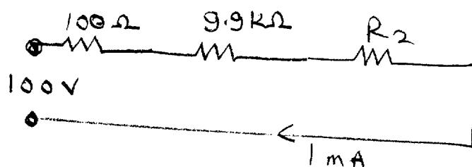
$$\begin{aligned} \therefore 100V &= (100 + 9.9 \text{ k}\Omega + R_2)(0.001) \\ &= (10,000 + R_2)(0.001) \end{aligned}$$
