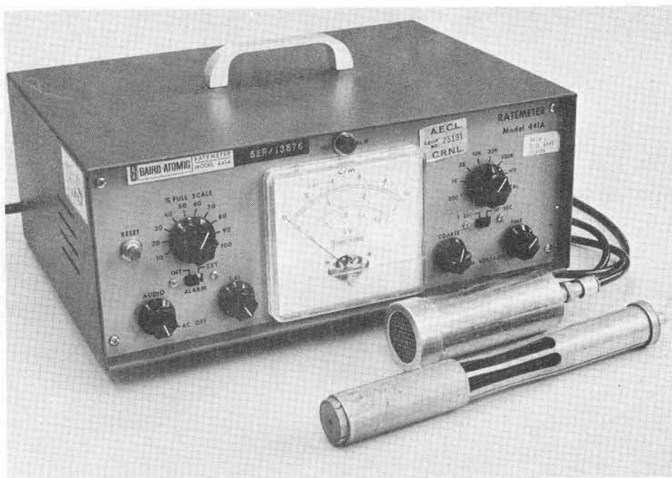
FIGURE 14 Baird Atomic Model 441A - AEP 4830 (Beta, Gamma)
