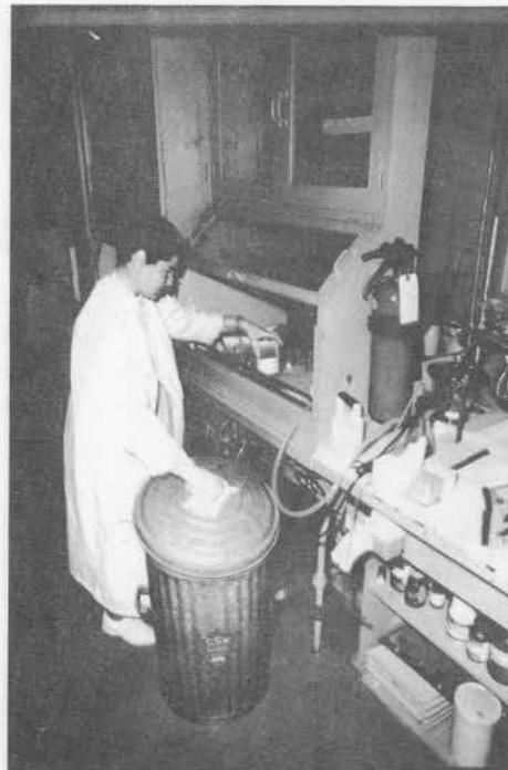
FIGURE 62 Active Waste Disposal Can
