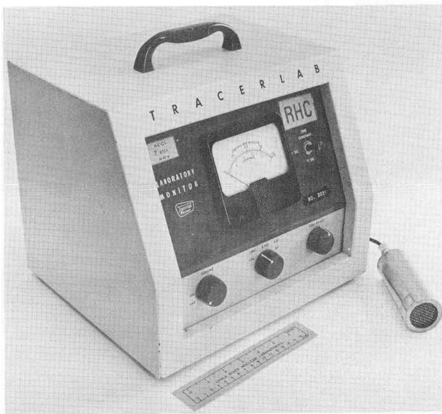
FIGURE 13 Tracerlab Model SU3D - AEP 1904 (Alpha, Beta, Gamma) (Alpha scintillation probe not shown)
