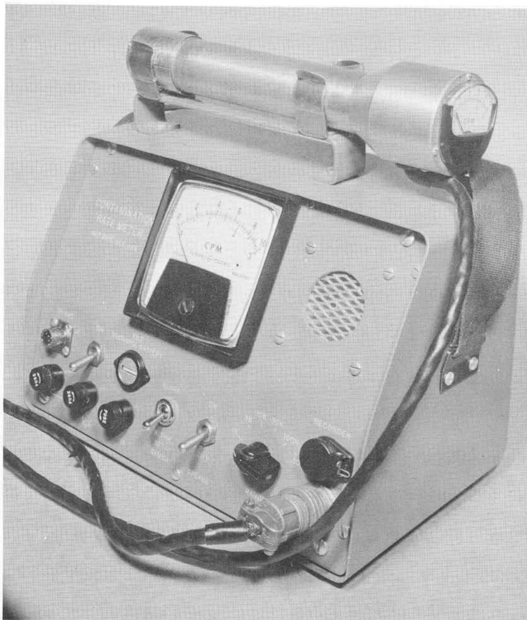
FIGURE 10 Contamination Ratemeter - AEP 2160 (alpha-Beta-Gamma)
