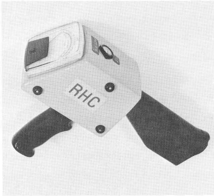
FIGURE 15 Multi-Purpose Survey Meter - AEP 2153A (Gamma)
