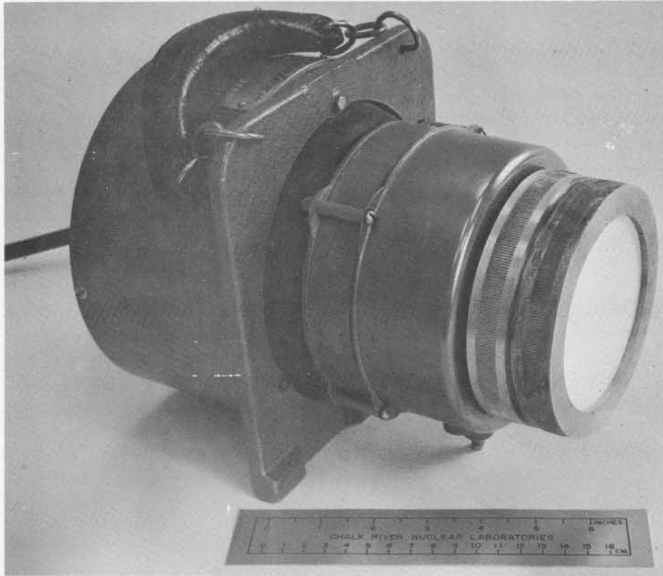
FIGURE 36 Staplex Sampler - GF/A Filter (Beta-Gamma)
