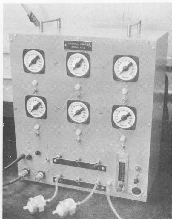
FIGURE 30 Sequential Air Sampler - May-Pack Iodine Filters
