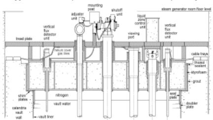
structure to provide a protected free space for cabling and services to the control units, while leaving an uncluttered walkway above for maintenance access. The tread plate also provides added local shielding during flasking operations to remove a device from the
