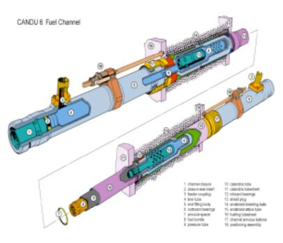
The pressure tube and end fittings are manufactured to the requirements of the ASME Boiler and Pressure Vessel Code, Section III, "Rules for Construction of Nuclear Power Plant Components", Subsection NB, "Rules for Class 1 Components" and form part of the primary heat transport system. The pressure tube has an inside diameter of about 104 mm, a wall thickness of about 4 mm and a length of about 6.3 m. The dissimilar metals of
