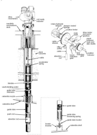
for a reactor trip and de-energizes the direct current clutches to release the absorber element portion of the shutoff units, allowing them to drop between columns of fuel channels, into the moderator. Each shutdown rod is equipped with a spring that provides an initial acceleration.
