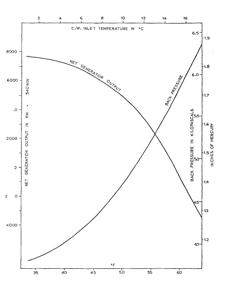
Effect of Cooling Water Temperature on Back Pressure and Net Output of Pickering G.S.
