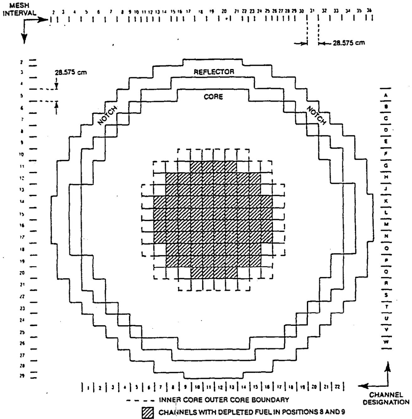
FIGURE 4.3-13 600 MW REACTOR MODEL FACE VIEW SHOWING INITIAL LOADING OF DEPLETED FUEL
