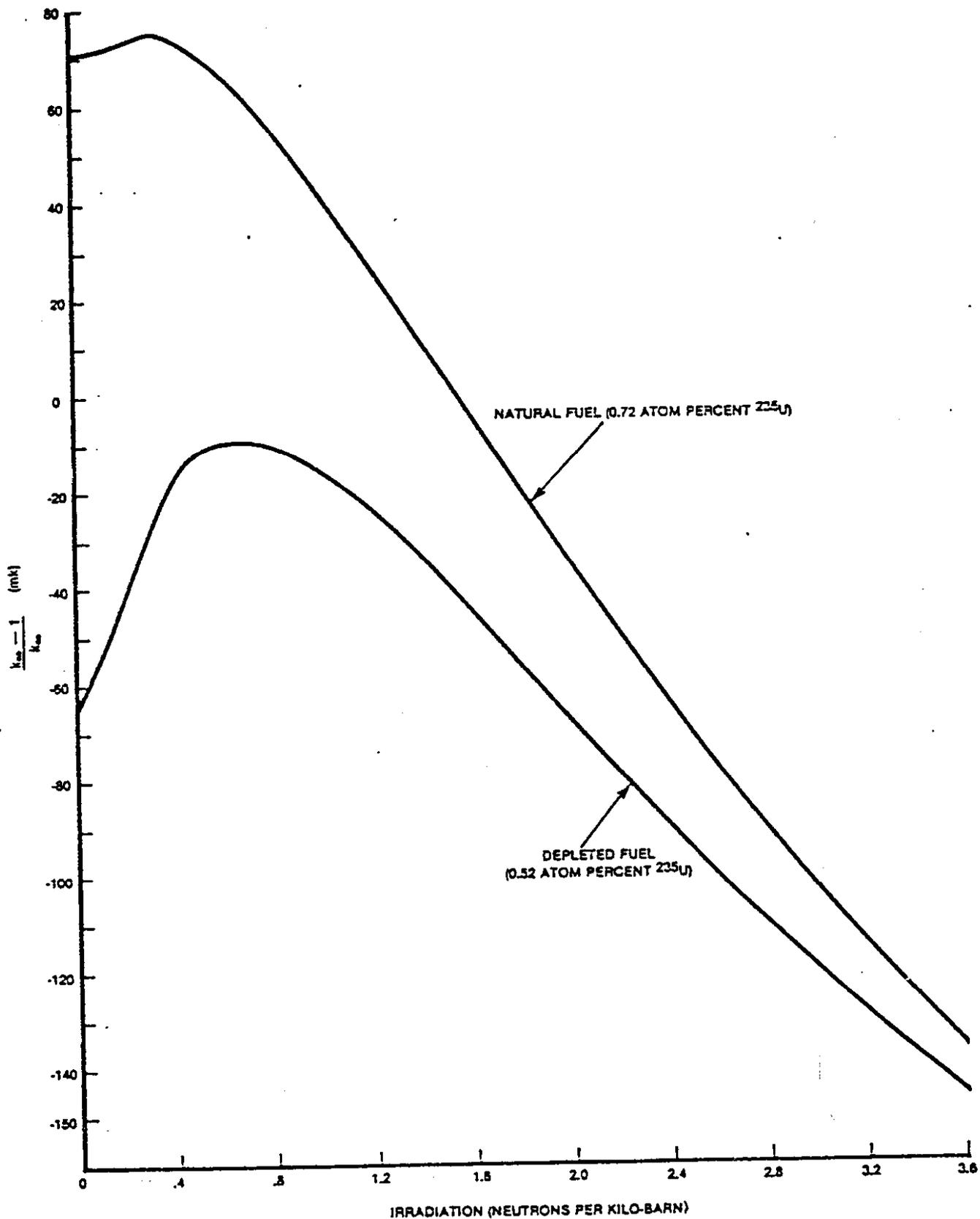
FIGURE 4.3-1 REACTIVITY OF 37-ELEMENT DEPLETED FUEL VERSUS IRRADIATION
