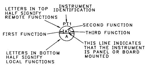
INSTRUMENTATION DEVICE, PANEL OR BOARD MOUNTED WITH INDICATION ON CONTROL ROOM PANEL OR OTHER REMOTE PANEL
