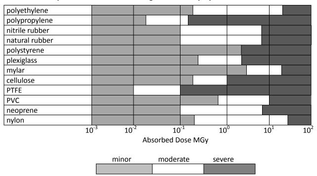
Table 4. Severity of radiation-induced damage of common polymers
