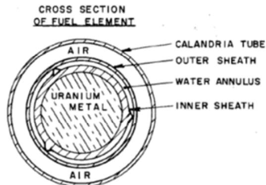
Figure 13 NRX fuel cross section
