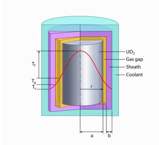
**Figure 65 Temperature distribution across a fuel pin**
