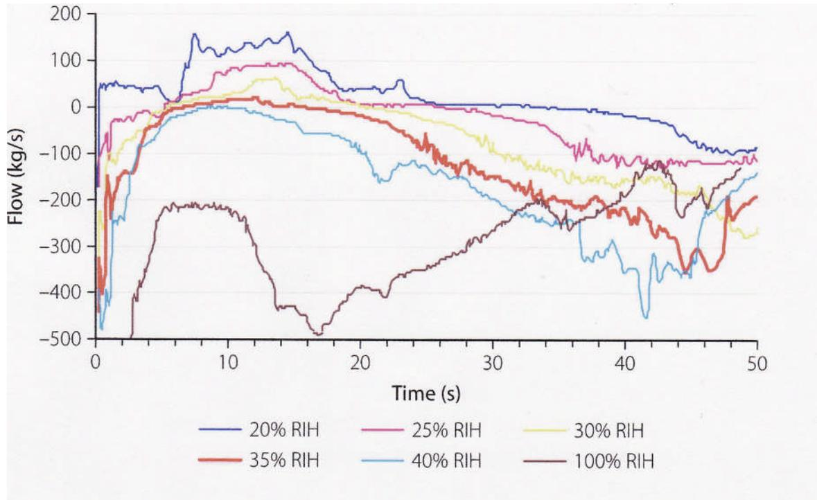
**Figure 54 Core flow vs. break size for a group of channels**
