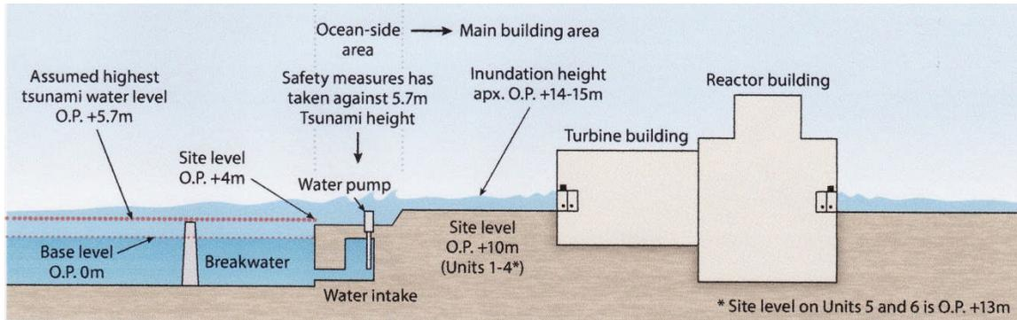
**Figure 23 Design basis versus actual flood level**
