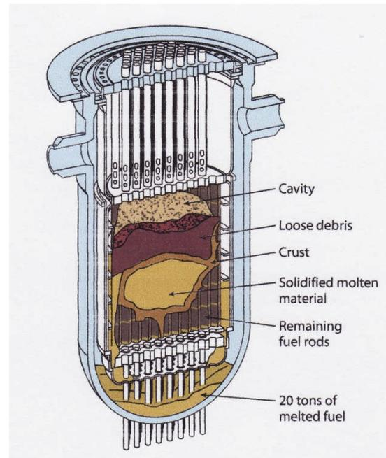
**Figure 20 TMI core end state**
