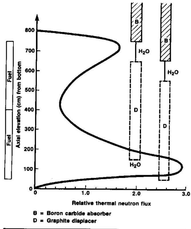
Figure 17 Reverse shutdown in RBMK
