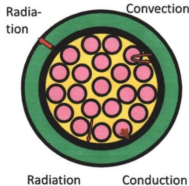
**Figure 67 Heat transfer to pressure tube**
