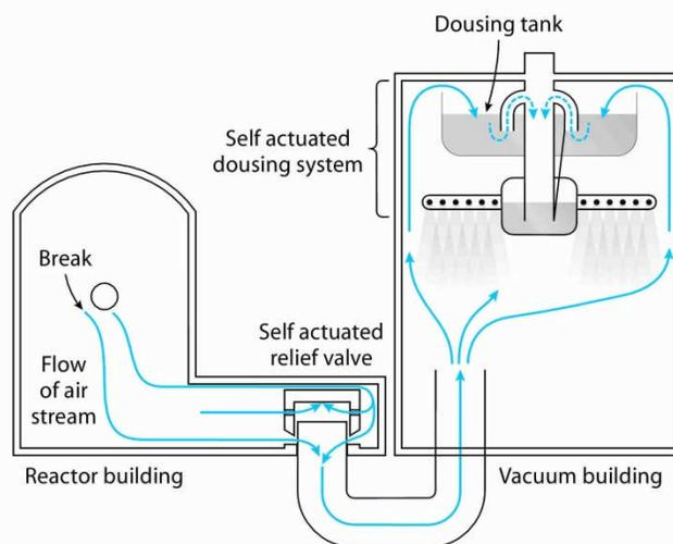
**Figure 43 Vacuum containment concept**
