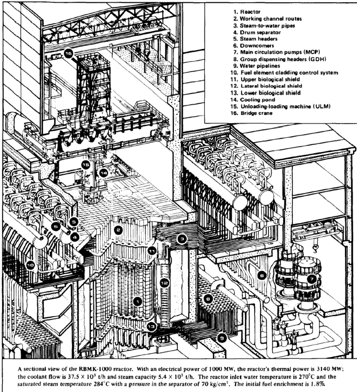
Figure 16 RBMK reactor
