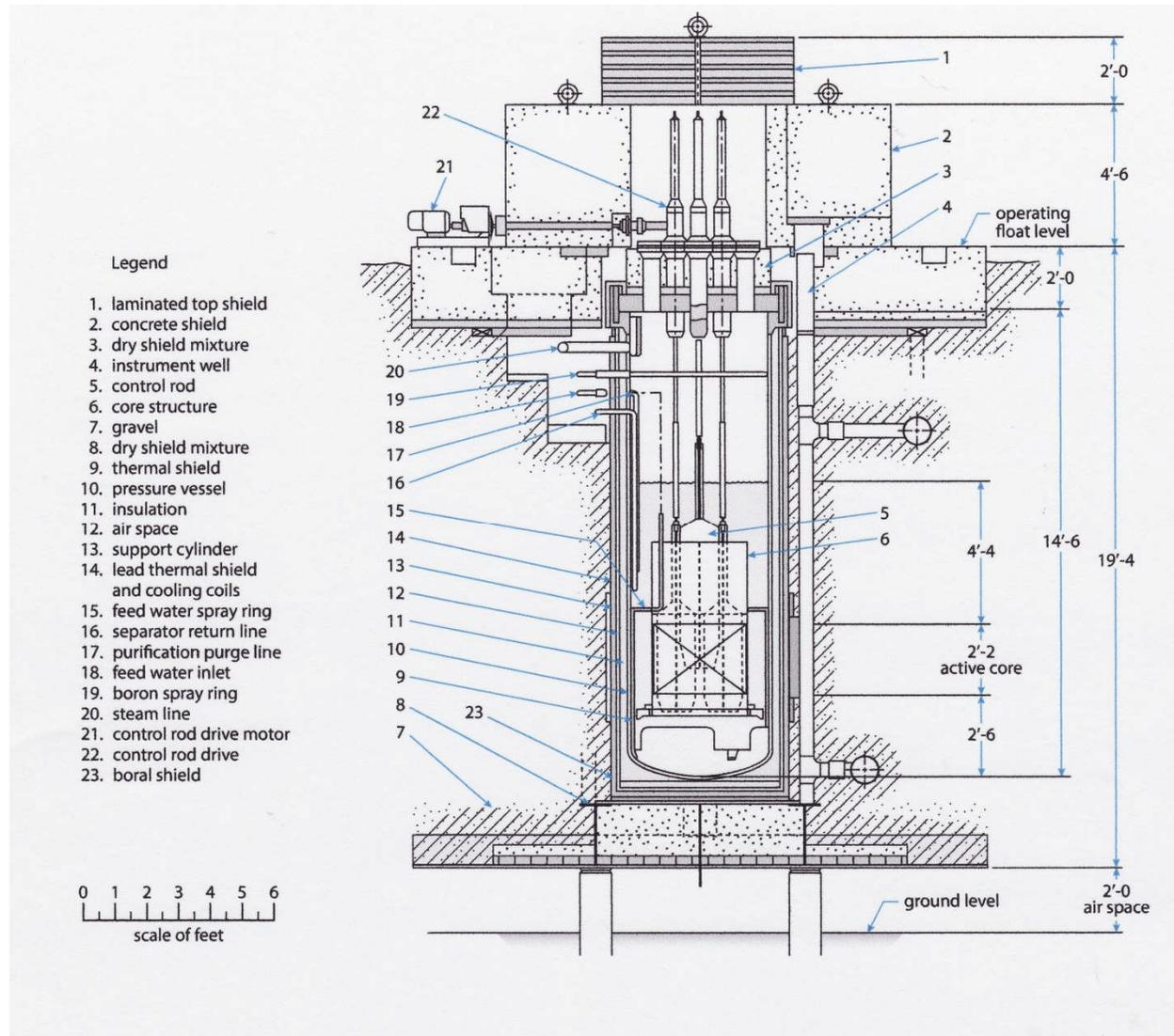
Figure 12 SL-1 cutaway
