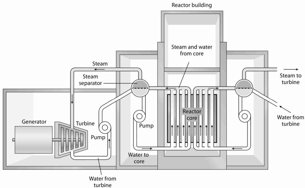
**Figure 18 RBMK building cross section**
