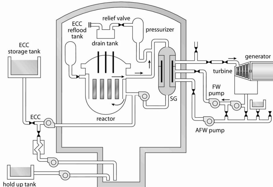
**Figure 19 TMI schematic**
