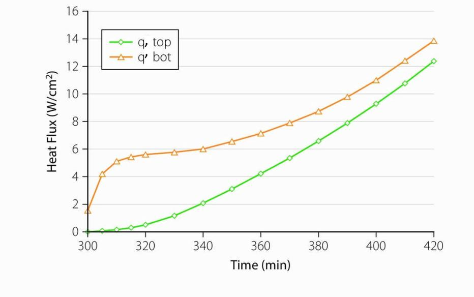
**Figure 64 Heat flux on calandria wall**
