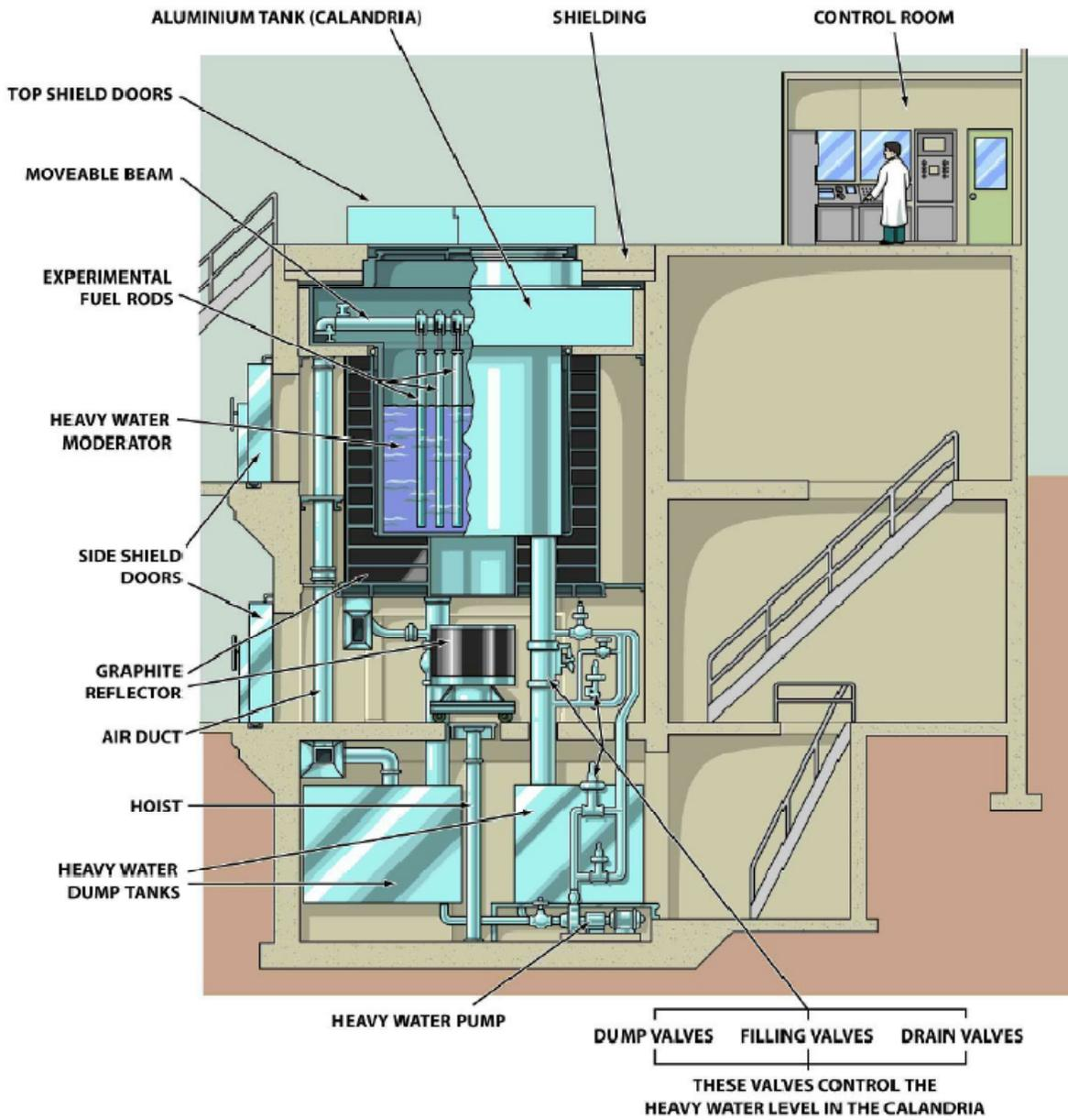
Figure 9 ZED-2 cutaway
