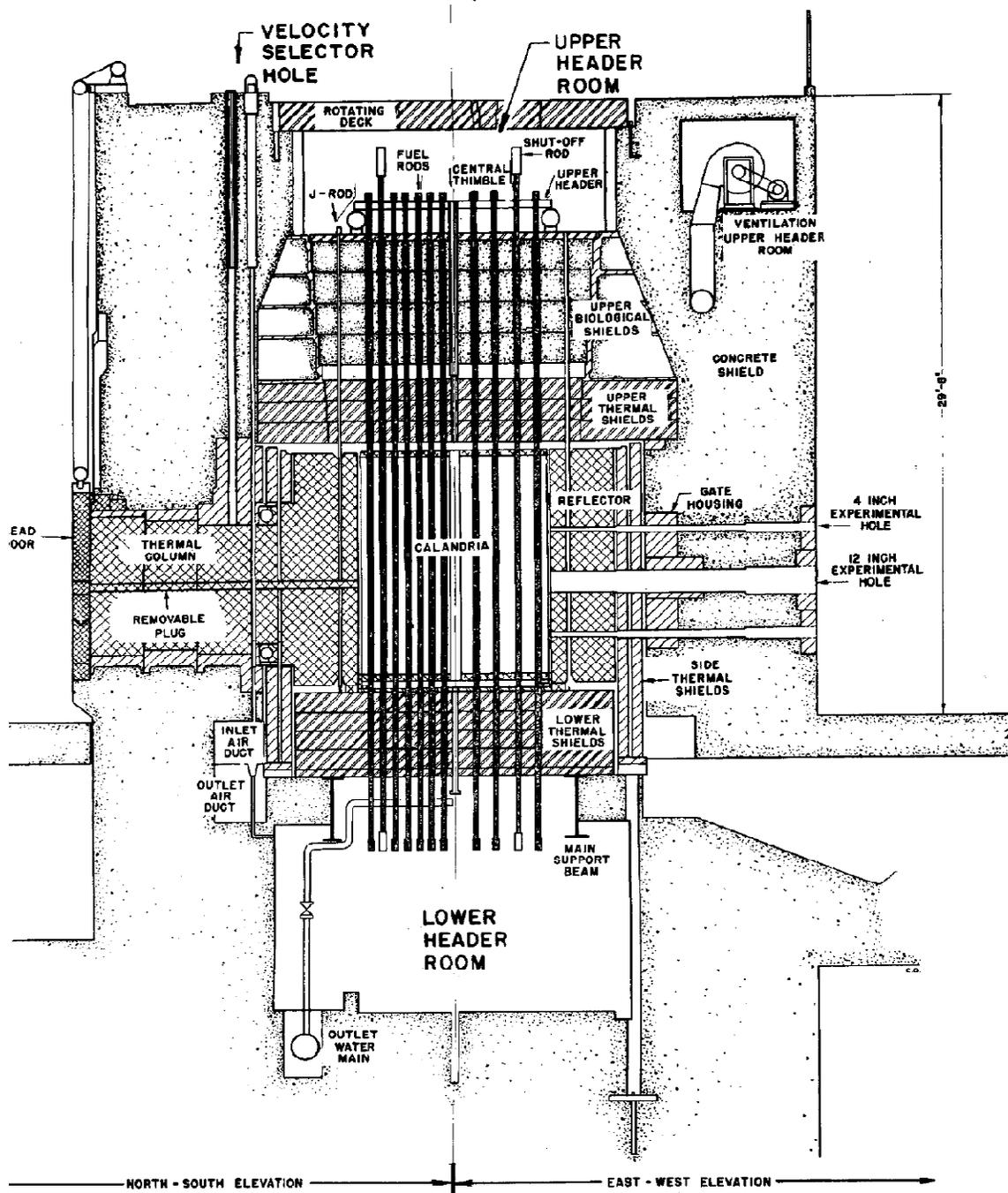
Figure 14 NRX elevation
