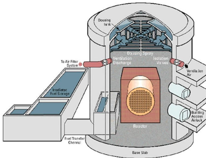
**Figure 42 Single-unit containment**
