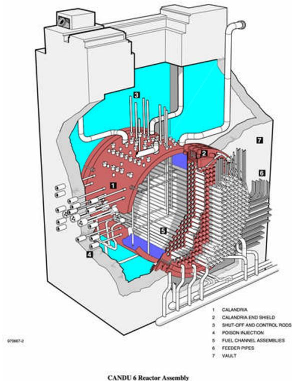
**Figure 39 Moderator and shield cooling**
