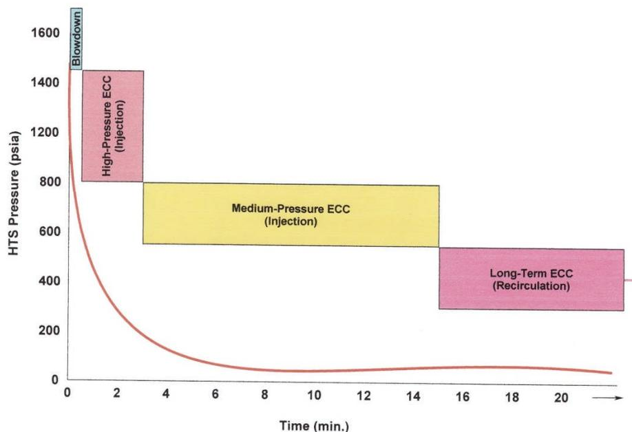
**Figure 41 Three phases of ECC**
