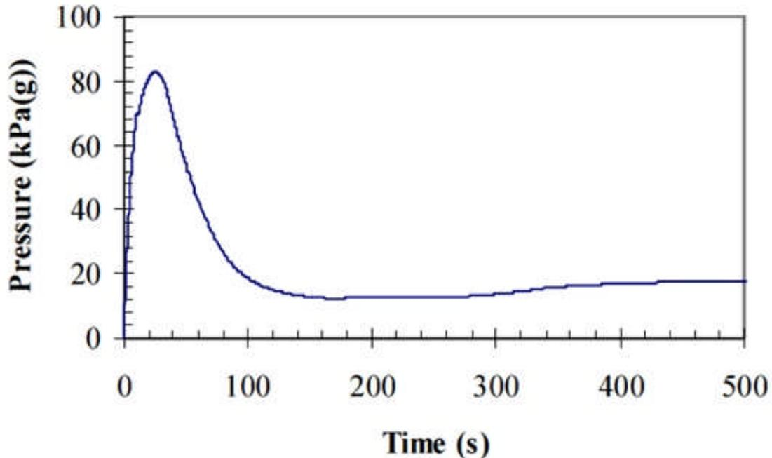
Figure 56 Containment pressure transient for 100% ROH LOCA
