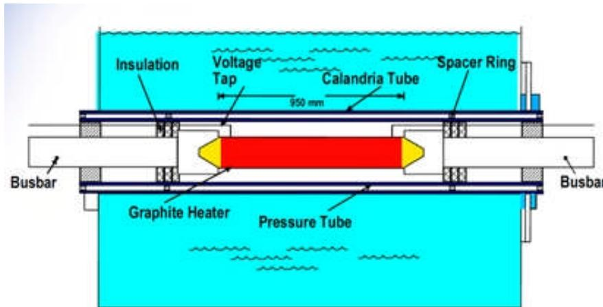
**Figure 48 Contact boiling tests**
