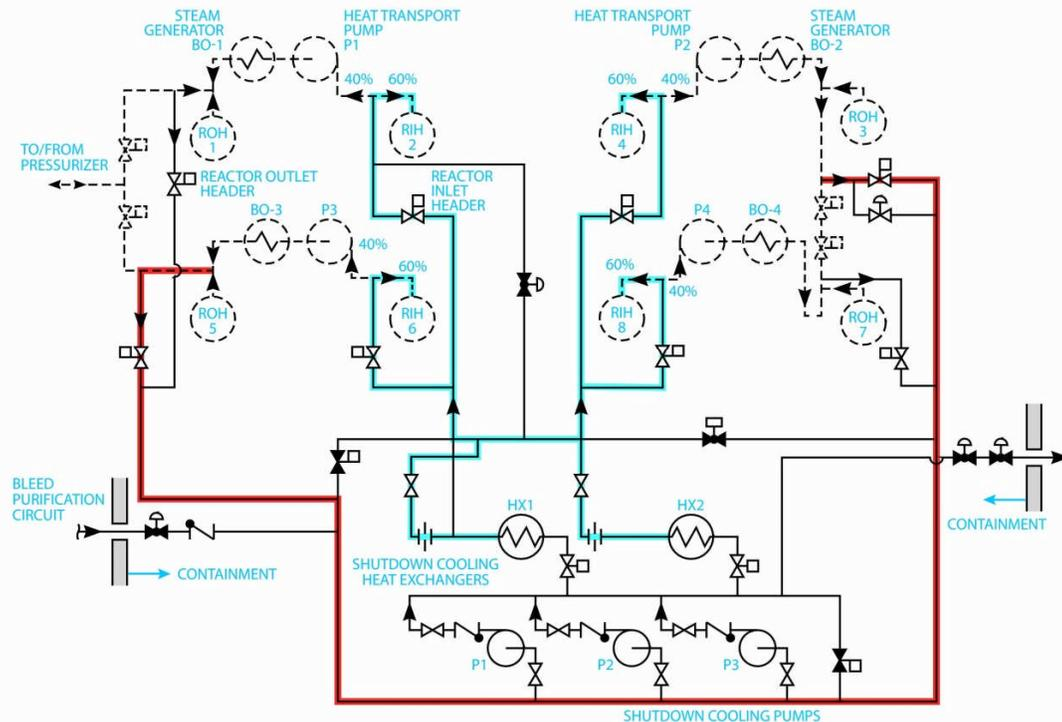
**Figure 38 Shutdown cooling system**
