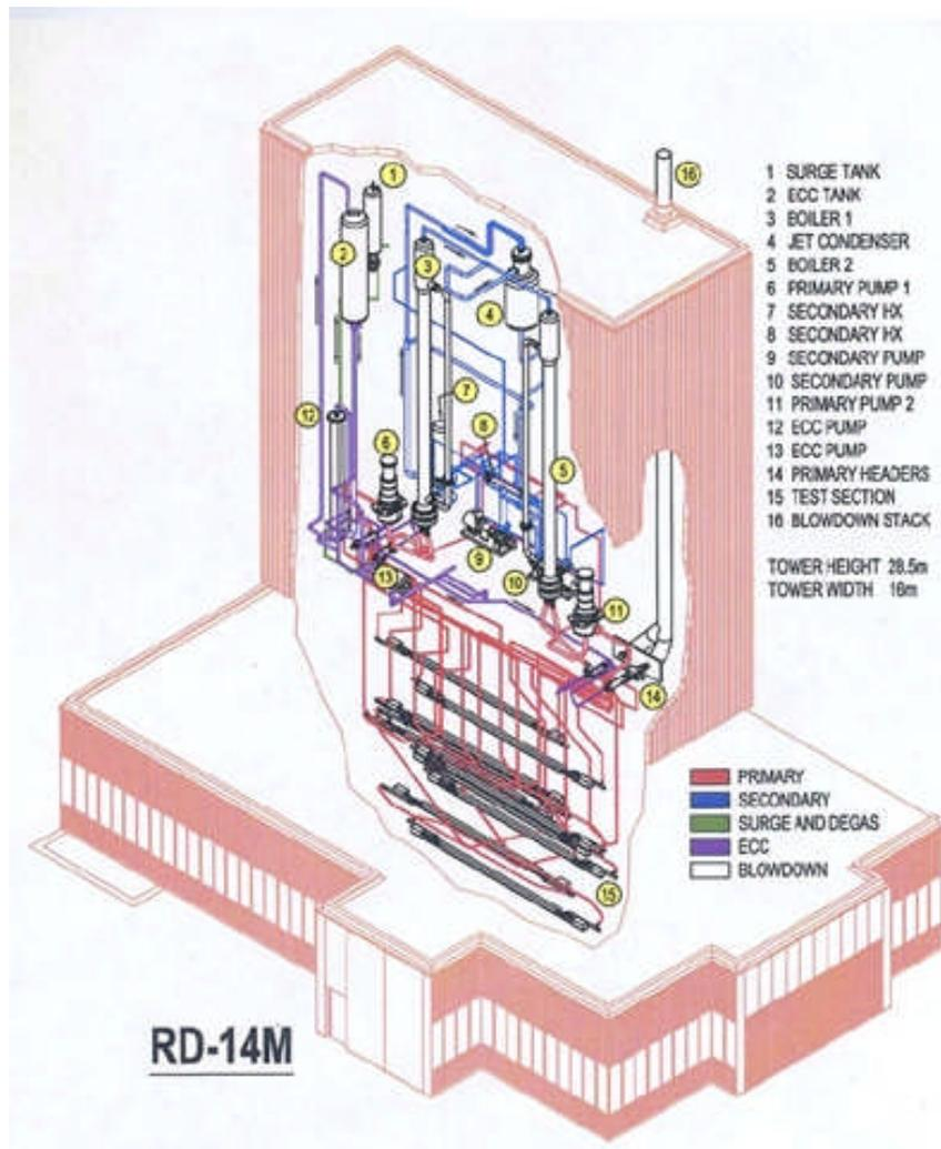
Figure 47 RD-14M schematic
