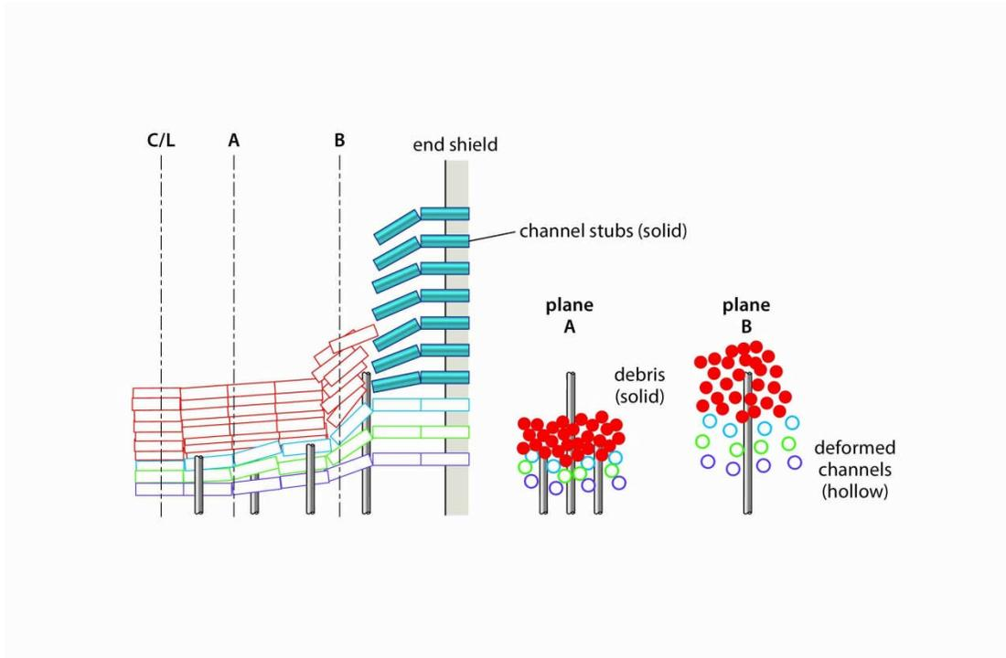
**Figure 60 Channel collapse in severe core-damage accident**
