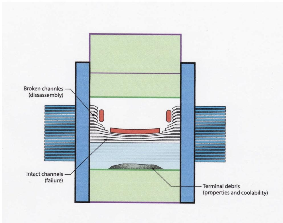
**Figure 61 Core collapse**
